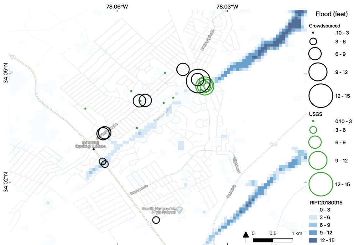
Figure 11. Comparison of flood depth in Boiling Spring Lakes, SC.
