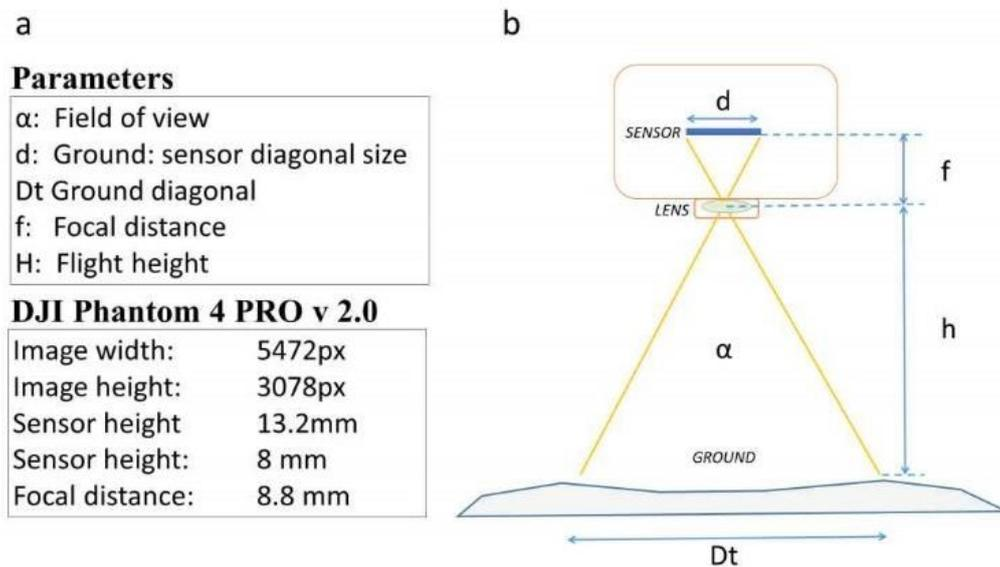
**Figure 2.** (a) Sensor characteristics of the DJI Phantom 4 PRO v 2.0; (b) parameters for calculating the distance of the sample to the ground: sensor diagonal size ( $d$ ), focal distance ( $f$ ), field of view ( $\alpha$ ), ground diagonal ( $Dt$ ), and vertical ground distance or flight height ( $h$ ). With this choice, a spatial resolution of 0.01–0.03 m was obtained, which was sufficient to recognize the smallest macro beached marine litter (BML).
