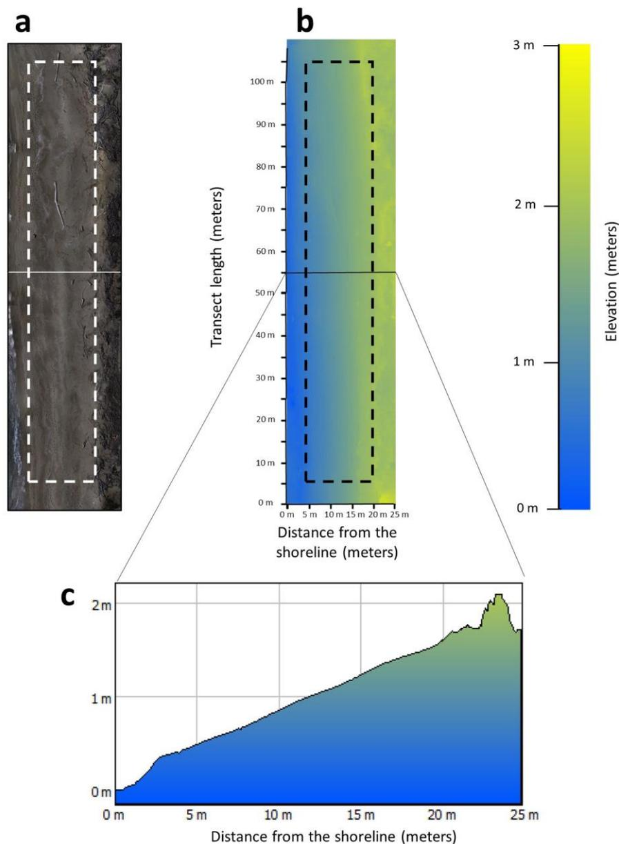
**Figure 5.** Orthophoto (a) and digital elevation models (DEM) (b) of the study area, with the profile of the beach corresponding to the central point of the sampled transect (c). Distances and elevation are indicated in the image, with the dotted line that delimits the study area inside the beach.
