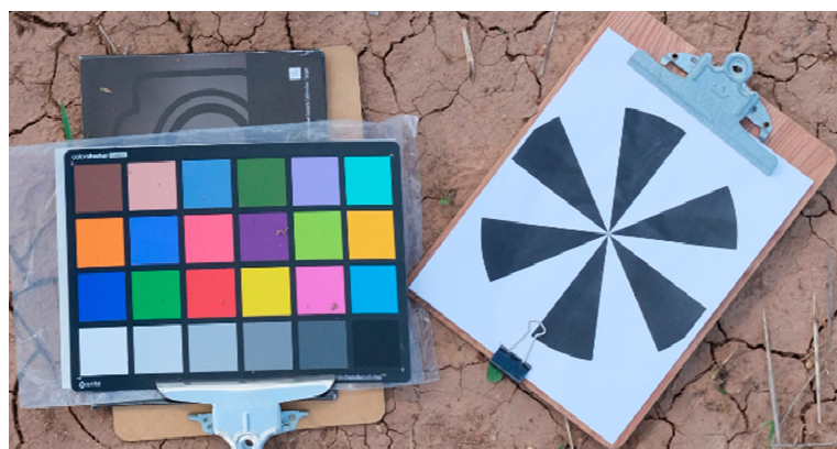
Figure 3. An example of the ColorChecker and the slant edge landmark image taken by the camera before data collection in the field, for estimating color transformation matrix M and point spread function (PSF).
