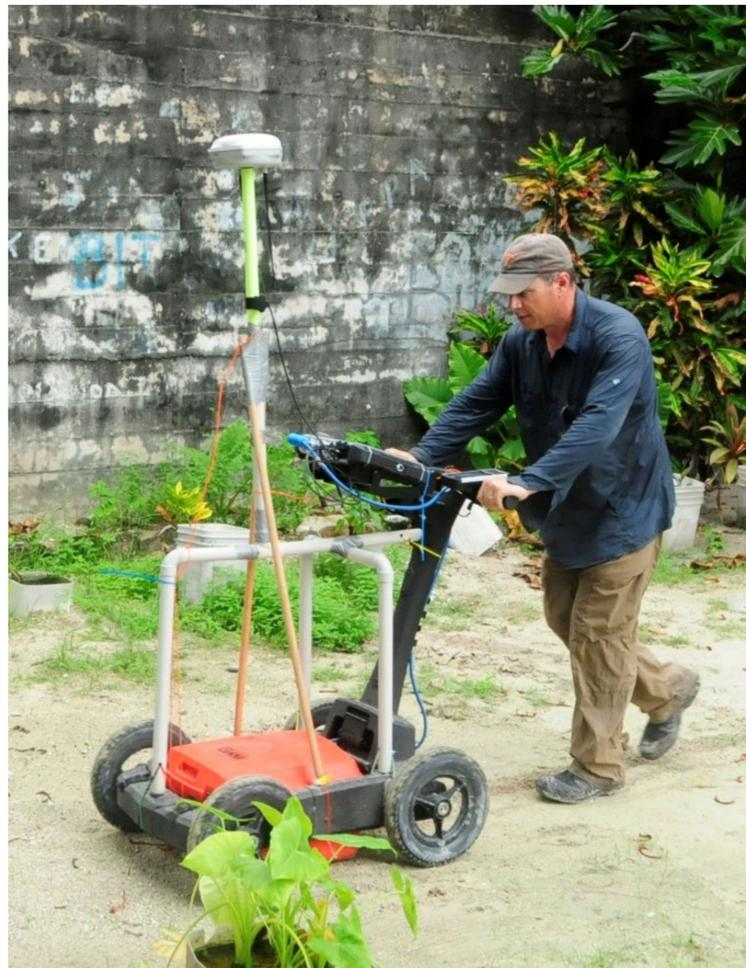
**Figure 1.** Typical GPR unit in use. GSSI SIR 4000 GPR with a 400 MHz antenna.
