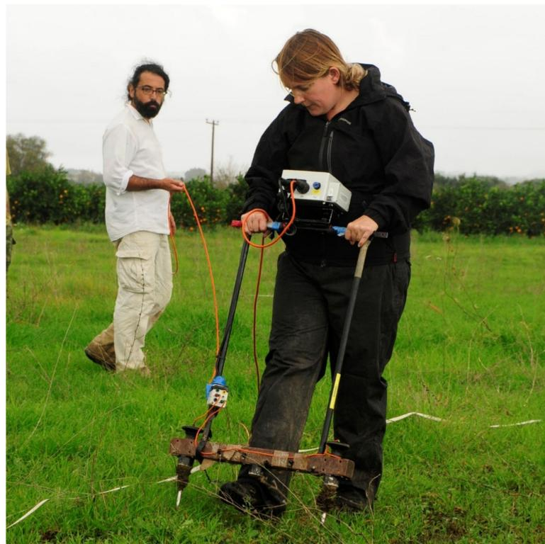
**Figure 3.** Geoscan Research RM85 Resistance Meter being used in the field.
