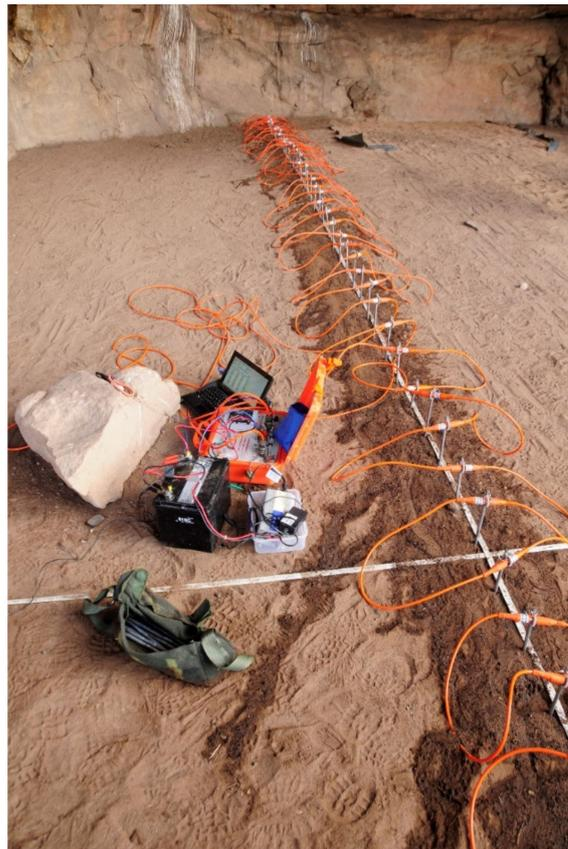
**Figure 2.** ZZ FlashRes64 ERT system being used in the field. Note the wetness around the electrodes from where they were watered to lower the contact resistance.
