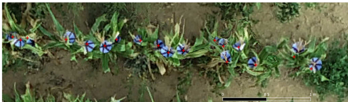
Figure 28. Final ortho-mosaic of R_1 reconstruction, visualized in the QGIS software, zoom on the second maize row, with in overlay the plant positions, measured on the ground with Geo7x DGNSS in pole mode (+).
