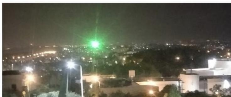
**Figure 7.** Terrestrial laser-beacon detection and tracking. A 0.002 Watt green laser as captured from ~9 km by a basic Raspberry Pi camera in VGA mode.
