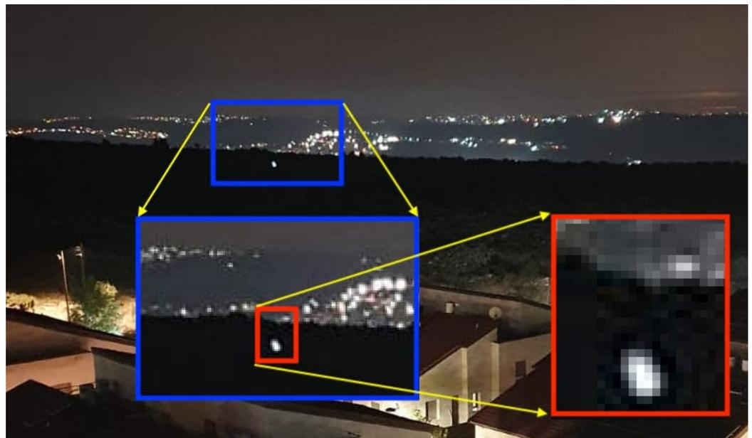
**Figure 9.** The LED array of SATLLA-2 (Eng-model) as seen from 1.1 km. The image was taken with a standard 70-degree smartphone camera—shooting at 30 fps in 1080p video format. It should be noted that in low-light-pollution conditions (on clear nights), SATLLA2 can be detected from more than 10 km using a standard Raspberry Pi V3 camera (FoV = 80, Sony IMX519).
