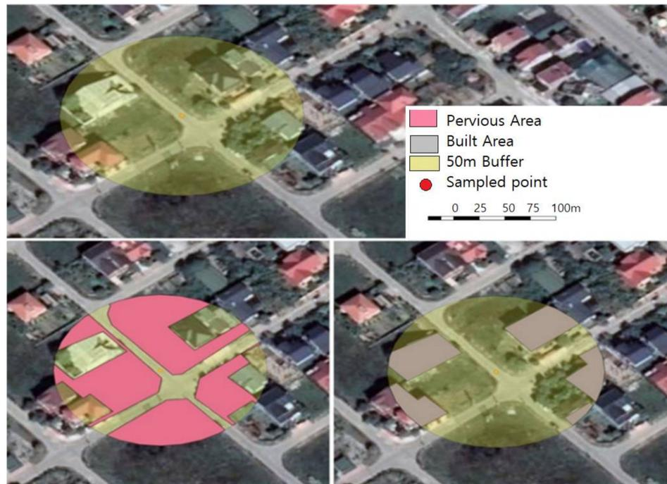
**Figure 4.** A display of the method for mapping the features within each polygon in order to classify it to the suitable LCZ [53].
