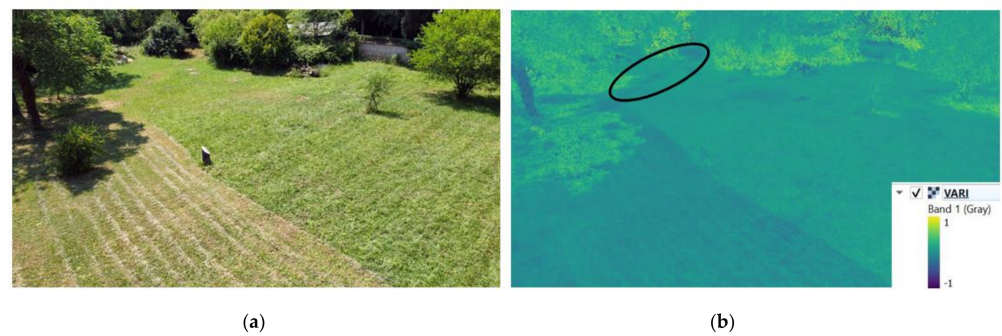
Figure 3. The comparison between visible and VARI images of the southern area of the garden: (a) The visible image; (b) The VARI image in which the presence of a possible manmade structure buried in the shallow subsurface is highlighted with a black circle.
