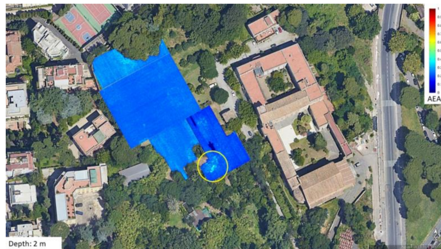
Figure 7. The GPR anomalies at 2 m (yellow circles).
