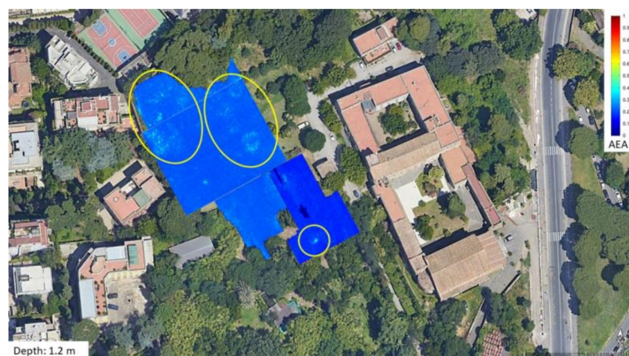
Figure 6. The GPR anomalies at 1.2 m (yellow circles).
