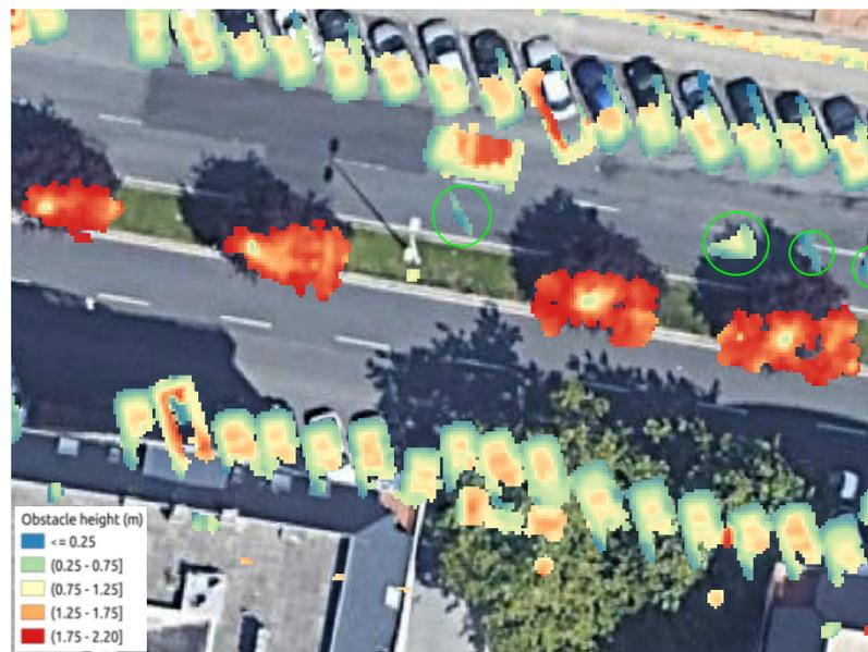
**Figure 8.** Height Above Ground (HAG) of the obstacles segmented as non-ground in the point cloud.
