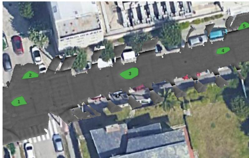
**Figure 7.** Occluded polygons. Example of Valle Inclán Street (A Coruña).
