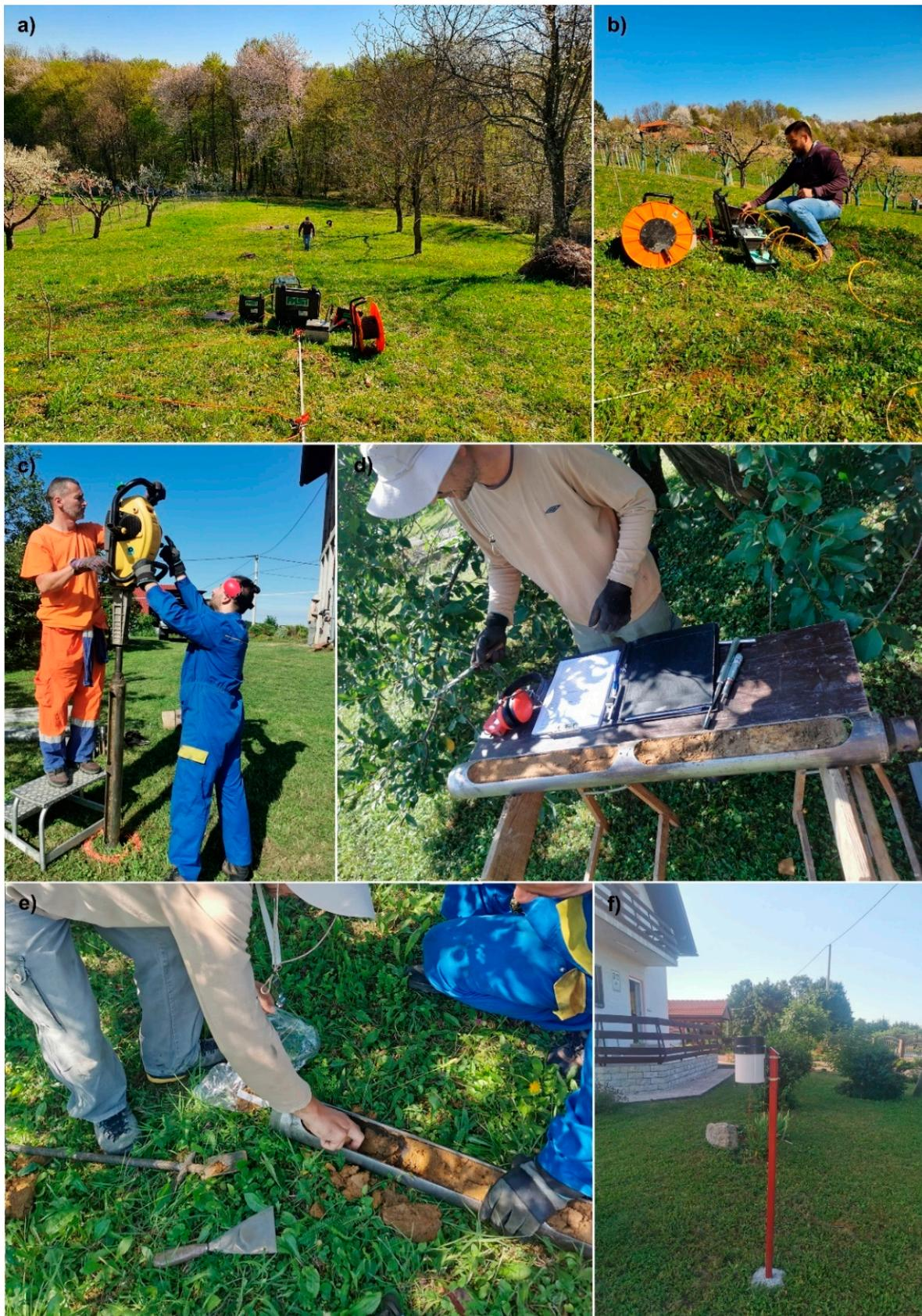
**Figure 3.** Overview of some field activities in Gajevo landslide area: (a) location of ERT3 cross-section outside landslide area; (b) measurement in progress on ERT3; (c) shallow borehole development; (d) borehole core determination; (e) borehole core sampling; (f) installed on-site pluviometer.
