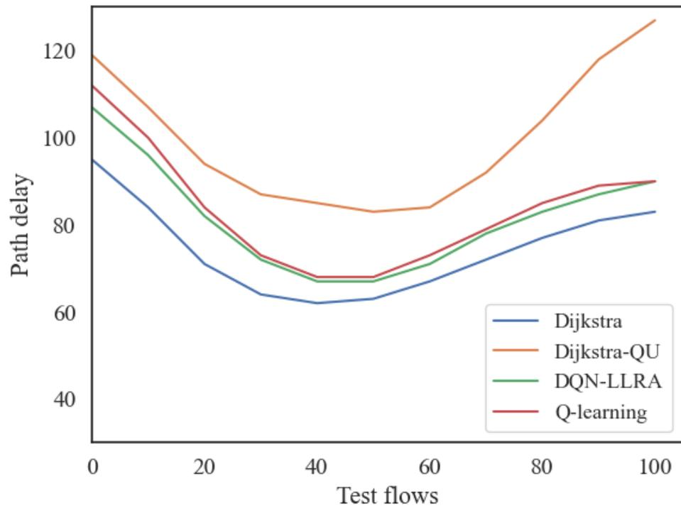
Figure 12. Path delay of different algorithms under various test flows.
