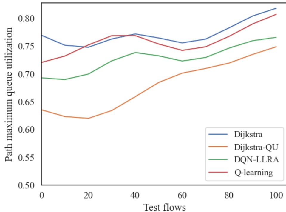
Figure 13. Path maximum queue utilization rates of different algorithms under various test flows.
