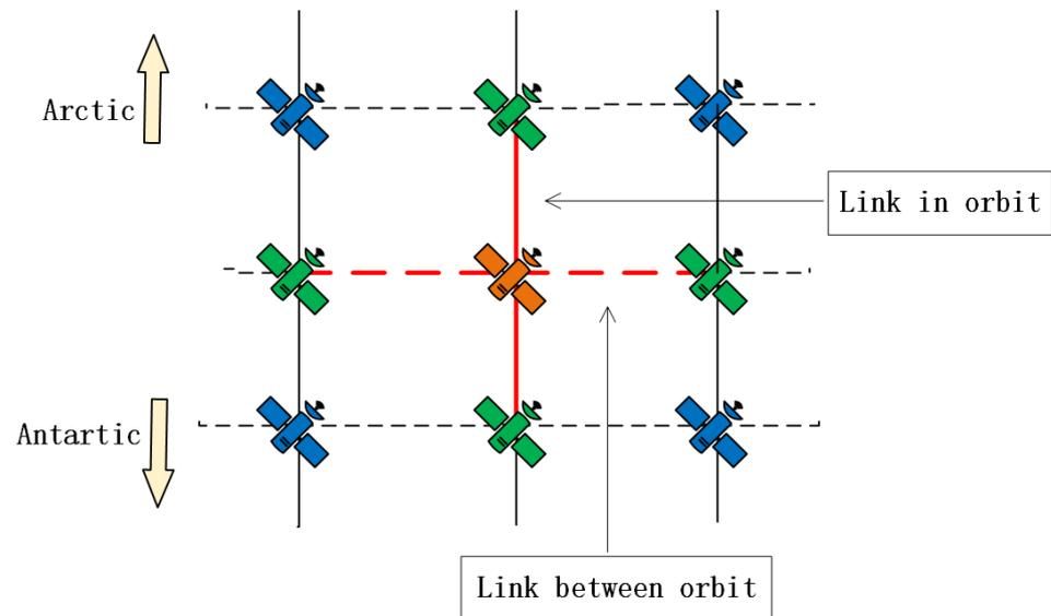
**Figure 4.** Schematic diagram of the inter-satellite links.
