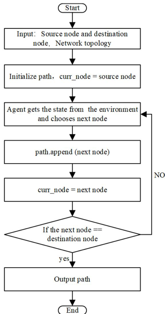
**Figure 7.** The decision flowchart of the DQN-LLRA algorithm.
