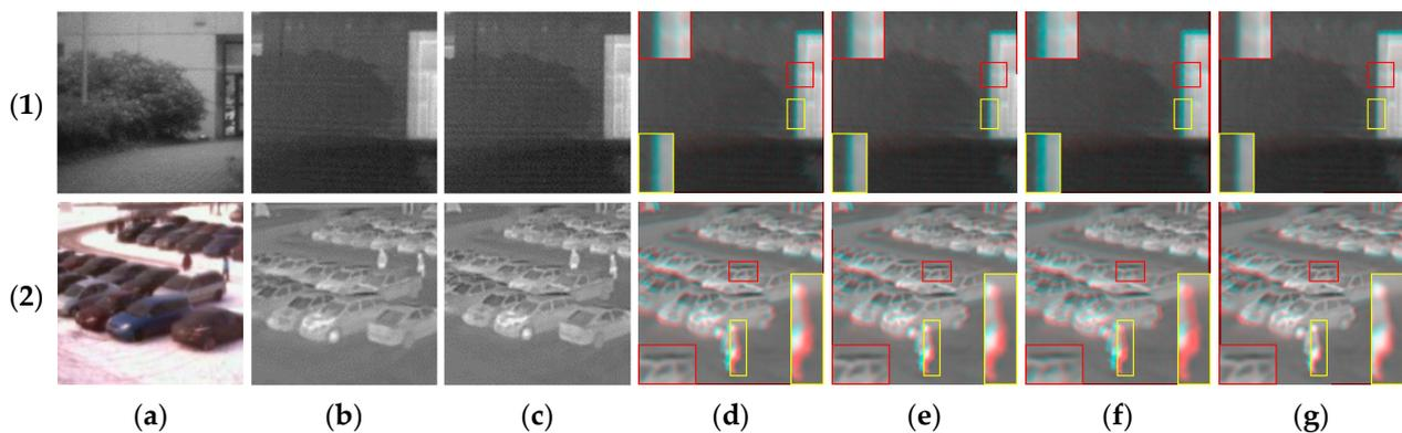
**Figure 8.** Comparison with the three deep learning-based methods in the two examples, as shown in (1) and (2). From left to right: (a) visible image; (b) infrared image; (c) ground-truth infrared image; (d) CADHN [43]; (e) DADHN [46]; (f) HomoMGAN [47]; and (g) the proposed algorithm. Error-prone regions are highlighted using red and yellow boxes, and the corresponding regions are zoomed in.
