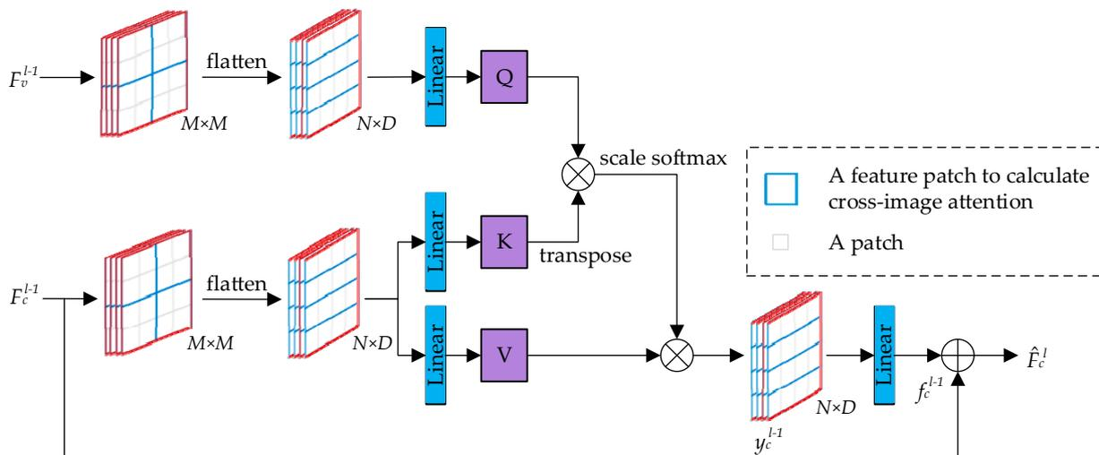
**Figure 5.** Network architecture of cross-image attention. Cross-image attention identifies the correlation between a feature patch in the source feature map and all feature patches in the target feature map within a window. The dimensionality of each feature patch is  $2 \times 2$ .
