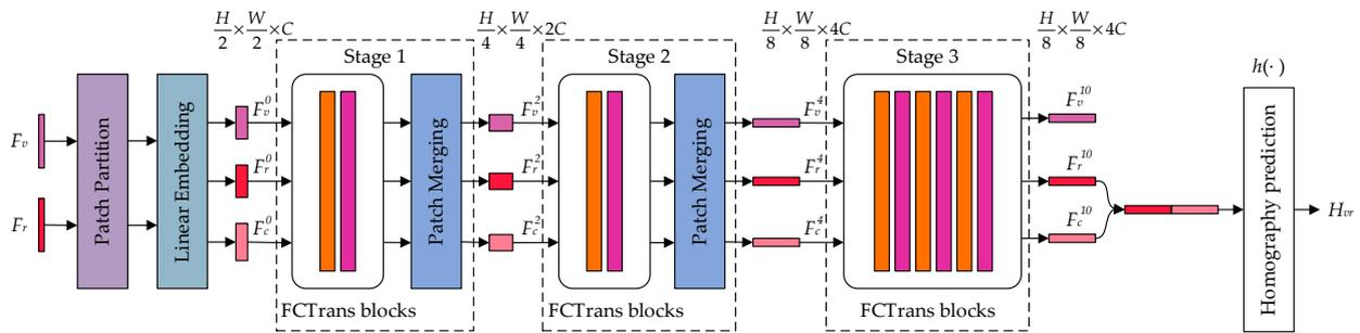
**Figure 3.** The overall architecture of the FCTrans. In the  $l$ -th FCTrans block, we consider  $F_v^l$  as the query feature map (source feature map),  $F_c^l$  as the key/value feature map (projected target feature map), and  $F_r^l$  as the reference feature map (unprojected target feature map).
