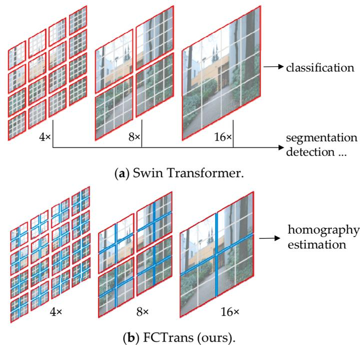
**Figure 1.** (a) The Swin Transformer computes attention in the unit of pixels (shown in gray) in each local window (shown in red). (b) The proposed FCTrans computes attention in the unit of the feature patch (shown in blue),  $2 \times 2$  in size, in each local window (shown in red), thus efficiently capturing high-level semantic features and adapting to differences between multi-source images.
