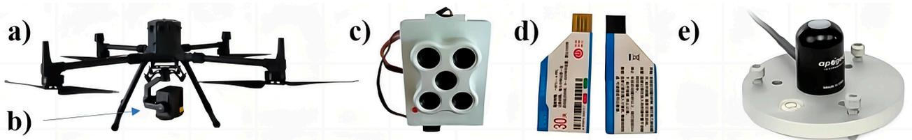
**Figure 2.** (a) DJI M300 RTK, (b) Zenmuse H20T thermal infrared camera, (c) RedEdge-MX five-channel multispectral camera, (d) temperature logger, (e) SP-110 solar total radiation sensor.
