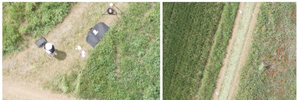
**Figure 8.** The three targets, of  $32 \times 32$  cm dimension, used to confirm the accuracies of the Agisoft Metashepe<sup>®</sup> resolutions.
