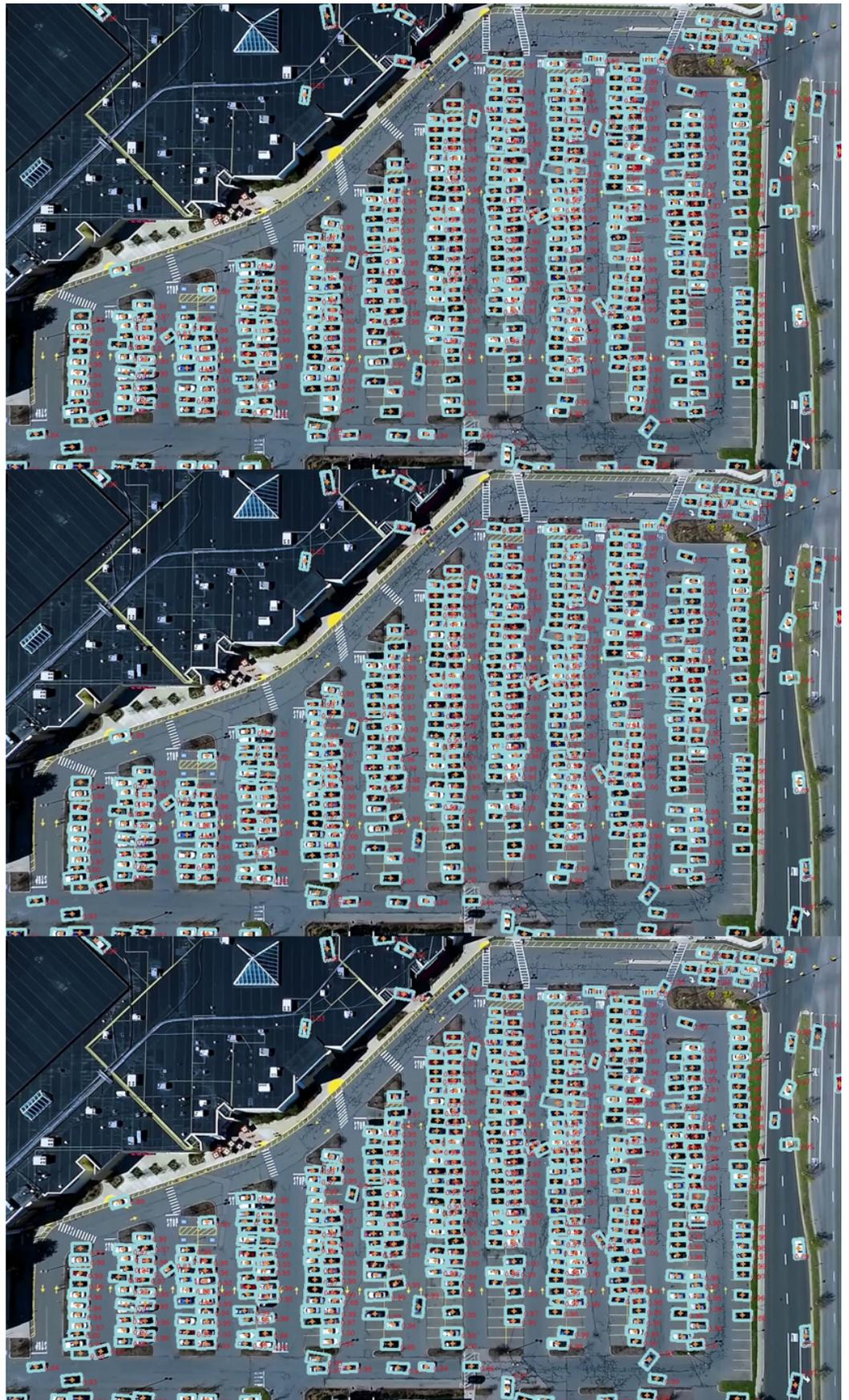
**Figure 11.** Detection result from aerial video frames without training. **Top:** frame-A; **second:** frame-B; **bottom:** frame-C.
