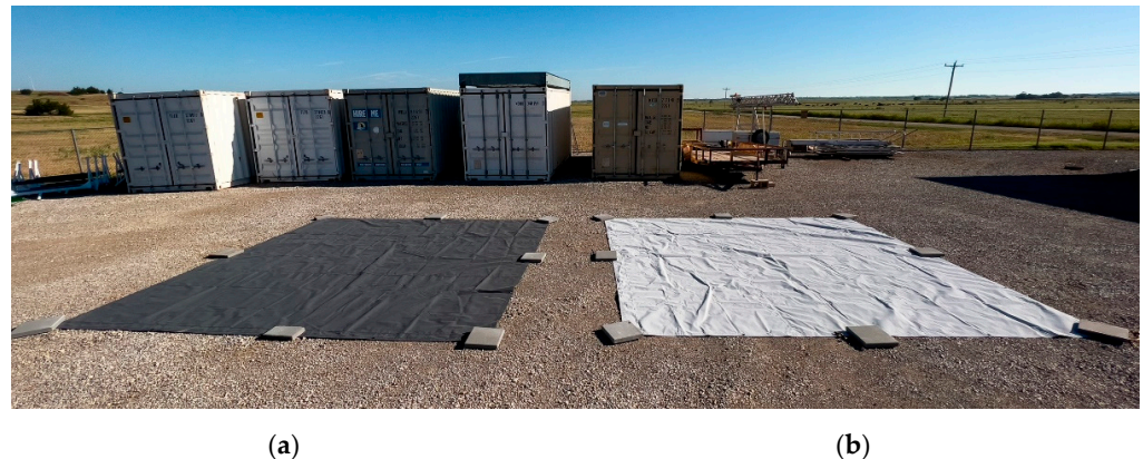
Figure 2. Field deployment of dark (a) and bright (b) calibration tarps with 11% reflectance and 48% reflectance, respectively.
