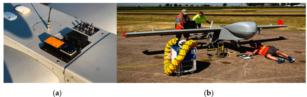
Figure 1. (a) The DLS2 installed on the dorsal hatch of the ArcticShark. The Altum imager is installed on a 3D-printed bracket mount in the payload bay (not pictured). (b) The challenges of a pre-flight Altum calibration for a mid-sized UAS. The aircraft must be tilted for panel capture on the ground. Proper capture for calibration requires that the DLS light sensor and panel be in the same light. Often, the UAS cast a shadow on the panel. Instead, we chose to validate our measurements to large reflectance tarps deployed in the sample area.
