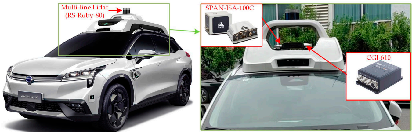
Figure 8. Shows the physical installation and arrangement of the autonomous driving platform vehicle and sensors.
