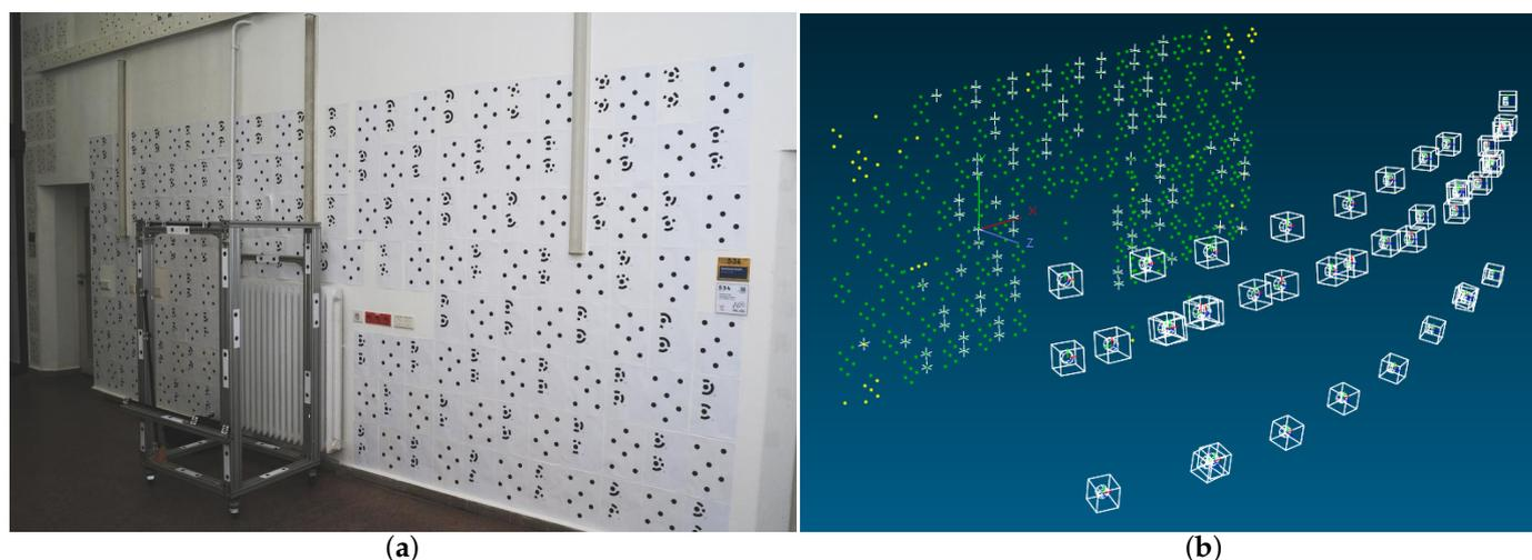
**Figure 5.** (a) Reference target field used for bundle adjustments. (b) Orientation of the images of the Panasonic Lumix DMC-GX80 camera and locations of the object points. The schematic illustration was created with the software package AICON 3D Studio (version 12.50.03).
