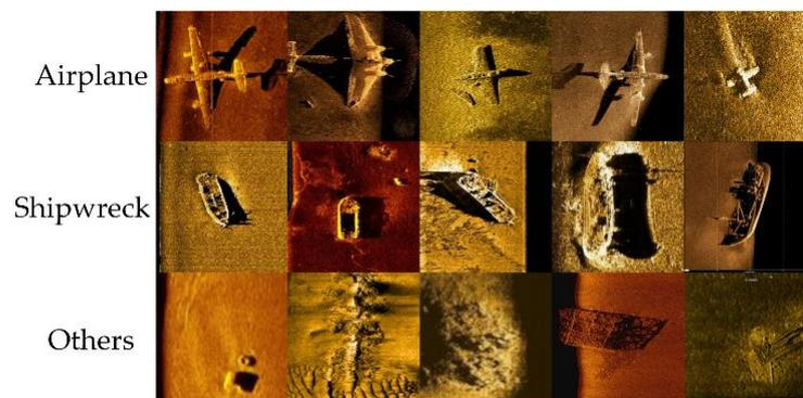
**Figure 14.** Examples of side-scan sonar image dataset.
