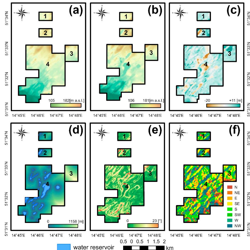
**Figure 8.** Independent variables—topographic factors: (a) DEM (1911); (b) DEM (2020); (c) DEM of Difference (2020–1911); (d) Distance from the anthropogenic lakes; (e) Slope of the terrain; (f) Aspect of the terrain.
