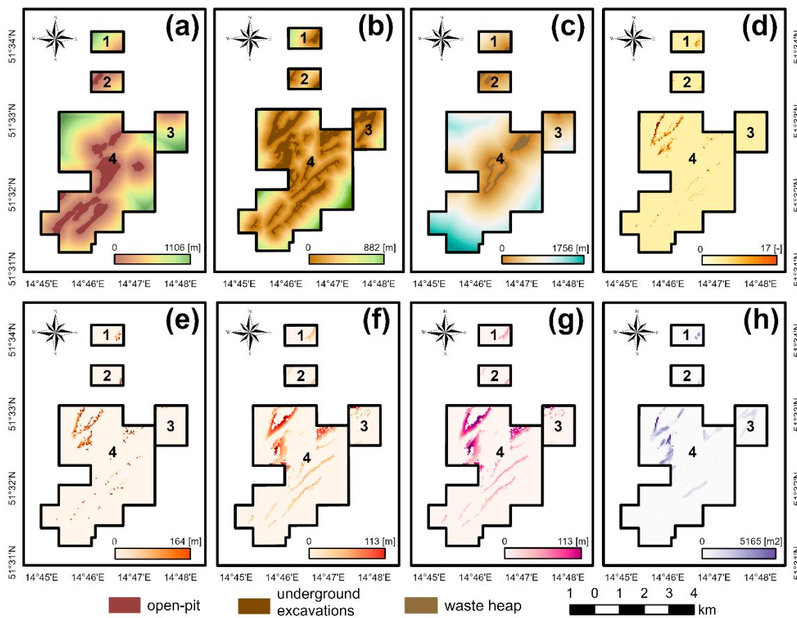
**Figure 6.** Independent variables—mining factors: (a) Distance from former open pits; (b) Distance from the underground workings; (c) Distance from the mining waste heaps; (d) Number of the mining shafts per pixel; (e) Average depth of the mining shafts; (f) Average depth of the underground excavations; (g) Minimum depth of the underground excavations; (h) Area of the underground mining excavations per 1 pixel.
