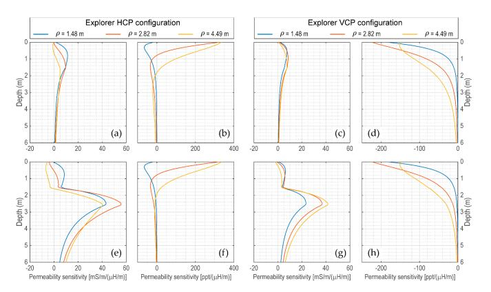
**Figure 16.** Sensitivity functions to magnetic permeability of the Explorer. (**a**,**c**) Q and (**b**,**d**) P sensitivities at 0.9 m above model M1; (**e**,**g**) Q and (**f**,**h**) P sensitivities at 0.9 m above model M2.
