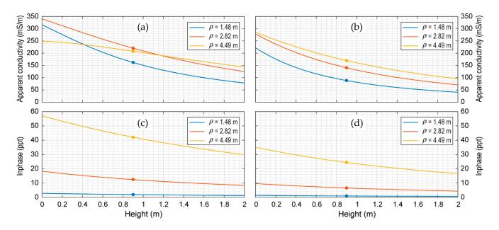
**Figure 10.** Electromagnetic response of the Explorer above the earth model M2. (**a**,**b**) are the simulated HCP and VCP quadrature (Q) responses, respectively, both expressed as apparent conductivity in mS/m; (**c**,**d**) are the HCP and VCP in-phase (P) responses, respectively. Dots indicate the response values at the probe height of 0.9 m, which is a frequently used operating height for both devices.
