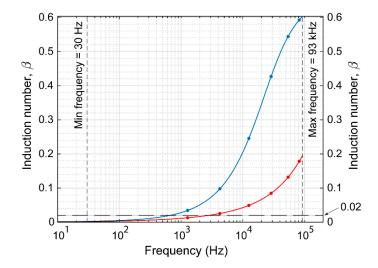
**Figure 12.** Induction numbers spanned over earth models M1 (red curve) and M2 (blue curve) by the full range of frequency available for the GEM-2. The horizontal dashed line at 0.02 indicates the transition from low to moderate induction numbers [80]. Dots indicate the induction numbers for a set of six selectable operating frequencies among those currently available for the GEM-2 (minimum frequency = 30 Hz; maximum frequency = 93 kHz).
