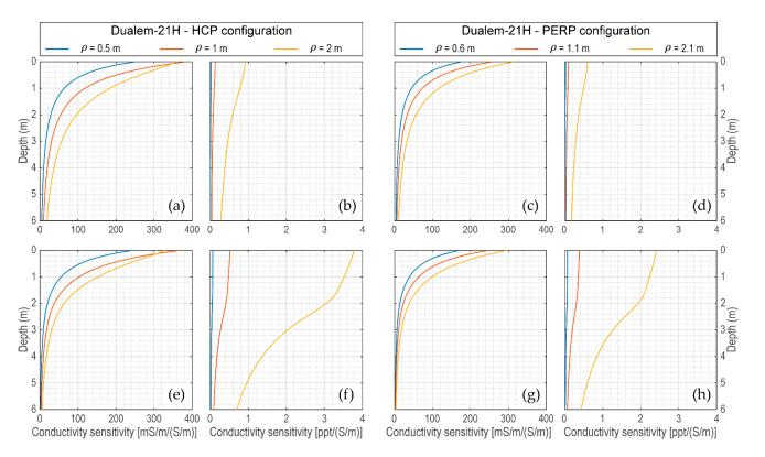
**Figure 13.** Sensitivity functions to electrical conductivity of the Dualem-21H. (**a**,**c**) Q and (**b**,**d**) P sensitivities at 0.9 m above model M1; (**e**,**g**) Q and (**f**,**h**) P sensitivities at 0.9 m above model M2.
