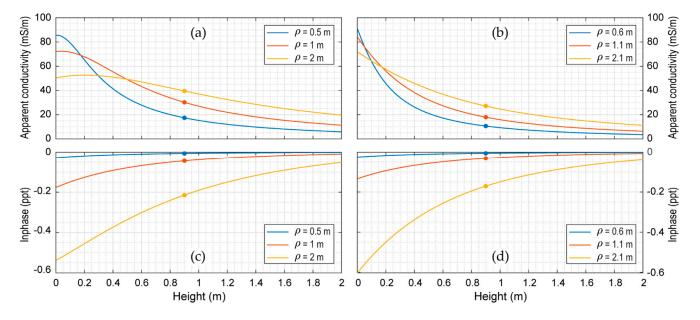
**Figure 7.** Electromagnetic response of the Dualem21H above the earth model M1. (a,b) are the simulated HCP and PERP quadrature (Q) responses, respectively, both expressed as apparent conductivity in mS/m; (c,d) are the HCP and PERP in-phase (P) responses, respectively. Dots indicate the response values at the probe height of 0.9 m, which is a frequently used operating height for both devices.
