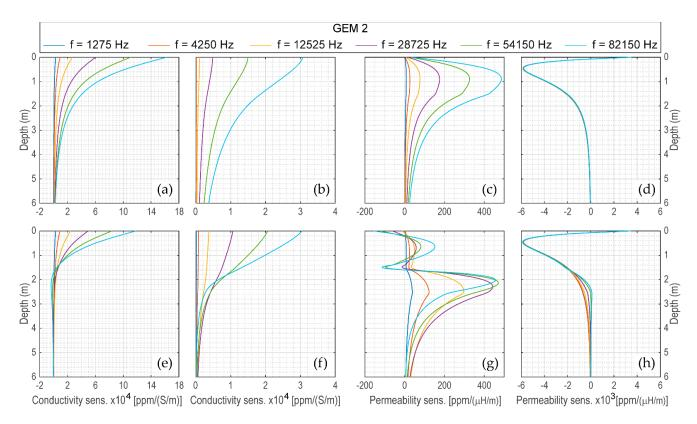
**Figure 17.** Sensitivity curves of the GEM-2. (**a**,**e**) Q and (**b**,**f**) P sensitivities to electrical conductivity at 0.9 m above models M1 and M2, respectively; (**c**,**g**) Q and (**d**,**h**) P sensitivities to magnetic permeability at 0.9 m above models M1 and M2, respectively.
