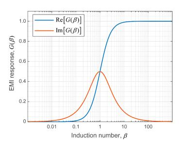
Figure A5. Real and Imaginary parts of the electromagnetic response function.
