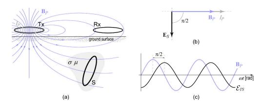
**Figure A2.** (a) Sketch of two magnetically coupled coils over a half-space with a conductive body. (b) Phasor diagram using as a reference the primary current. The secondary electric field lags the primary magnetic field by 90°. (c) Time dependence of  $\mathcal{E}_{TS}(t)$  and  $\mathbf{B}_P(t)$  that shows the same lagging phase as in the phasor diagram.
