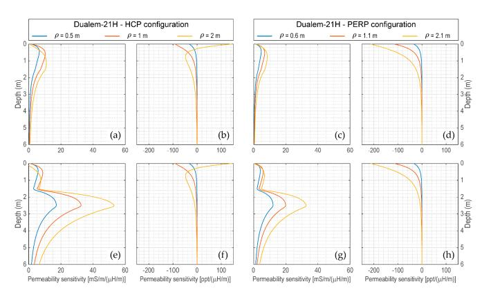
**Figure 14.** Sensitivity functions to magnetic permeability of the Dualem-21H. (**a**,**c**) Q and (**b**,**d**) P sensitivities at 0.9 m above model M1; (**e**,**g**) Q and (**f**,**h**) P sensitivities at 0.9 m above model M2.
