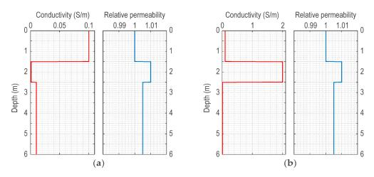
**Figure 6.** (a) Earth model M1; (b) earth model M2. Models differ only in the electrical conductivity of the middle layer.
