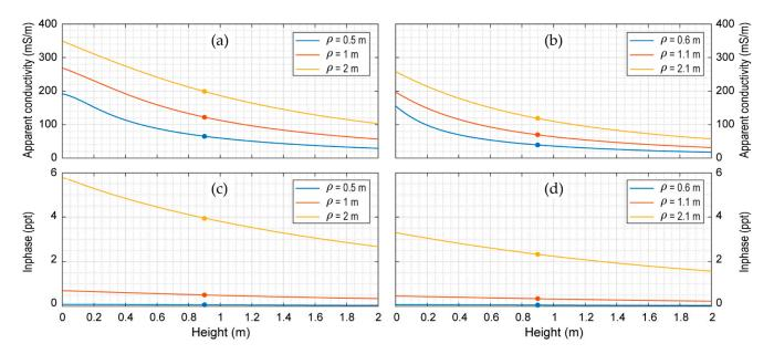
**Figure 9.** Electromagnetic response of the Dualem21H above the earth model M2. (**a**,**b**) are the simulated HCP and PERP quadrature (Q) responses, respectively, both expressed as apparent conductivity in mS/m; (**c**,**d**) are the HCP and PERP in-phase (P) responses, respectively. Dots indicate the response values at the probe height of 0.9 m, which is a frequently used operating height for both devices.
