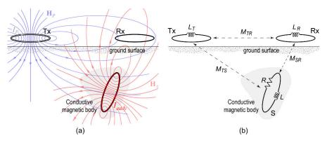
**Figure 2.** (a) Schematic full process of electromagnetic induction (modified from [7,44]); blue and red lines depict imaginary force lines of the primary and secondary magnetic fields, respectively. (b) Single-loop coupled *LR* equivalent circuits (modified from [44]);  $L_T$  and  $L_R$  are the self-inductance of coils Tx and Rx, respectively, while  $M_{ij}$ , with i, j = T, R, S, denotes the mutual inductance of any two of the coils.
