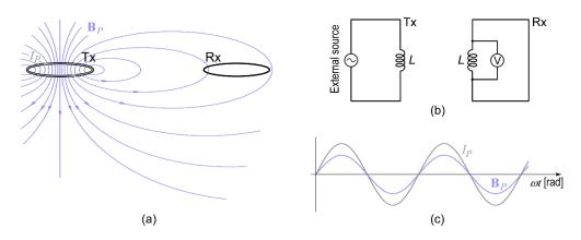
**Figure A1.** (a) Sketch of two magnetically coupled coils in a free space. (b) Equivalent single-loops circuits for the transmitter (on the left) and the receiver (on the right) coils. (c) Primary current and primary magnetic field as a function of time.
