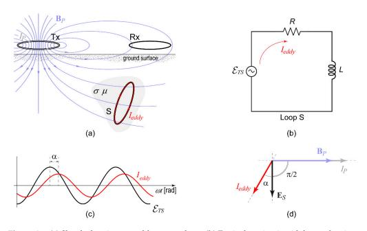
**Figure A3.** (a) Sketch showing one eddy current loop. (b) Equivalent circuit with lumped resistance R and inductance L, connected across an alternating voltage source. (c) Time dependence of  $\mathcal{E}_{TS}(t)$  and  $I_{eddy}(t)$  across loop S; the current lags the voltage. (d) Phasor diagram using as a reference the primary current. The secondary electric field lags by 90° the primary magnetic field, while eddy currents show an additional phase lag.
