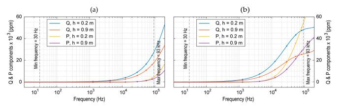
**Figure 11.** Electromagnetic response of GEM-2. (**a**) Quadrature and in-phase components of responses at heights of 0.2 and 0.9 m above ground surface of earth model M1; (**b**) Quadrature and in-phase components of responses at heights of 0.2 and 0.9 m above ground surface of earth model M2. Dots indicate the response values for a set of six selectable operating frequencies among those currently available for the GEM-2 (minimum frequency = 30 Hz; maximum frequency = 93 kHz).
