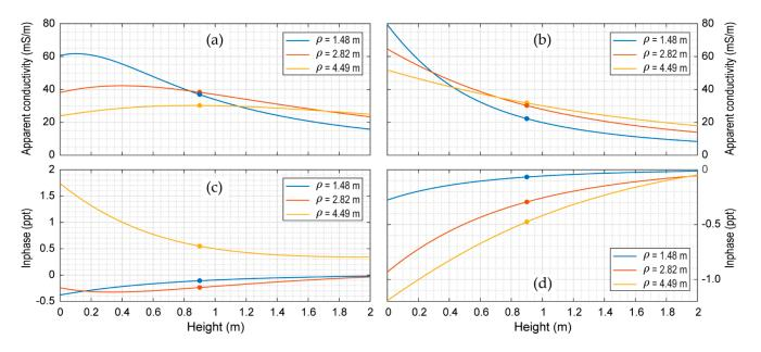
**Figure 8.** Electromagnetic response of the Explorer above the earth model M1. (**a**,**b**) are the simulated HCP and VCP quadrature (Q) responses, respectively, both expressed as apparent conductivity in mS/m; (**c**,**d**) are the HCP and VCP in-phase (P) responses, respectively. Dots indicate the response values at the probe height of 0.9 m, which is a frequently used operating height for both devices.
