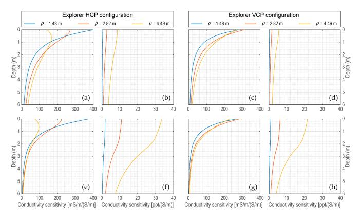
**Figure 15.** Sensitivity functions to electrical conductivity of the Explorer. (**a**,**c**) Q and (**b**,**d**) P sensitivities at 0.9 m above model M1; (**e**,**g**) Q and (**f**,**h**) P sensitivities at 0.9 m above model M2.
