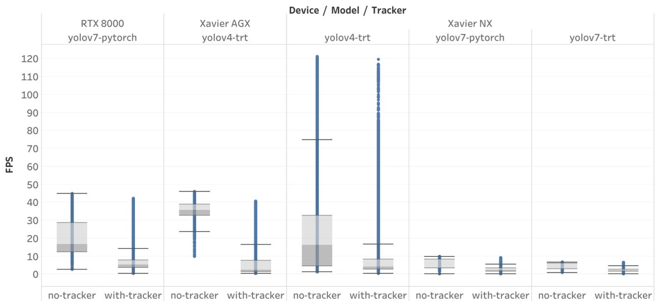
Figure 9. Inference speed per device, detection model, and use of tracker.
