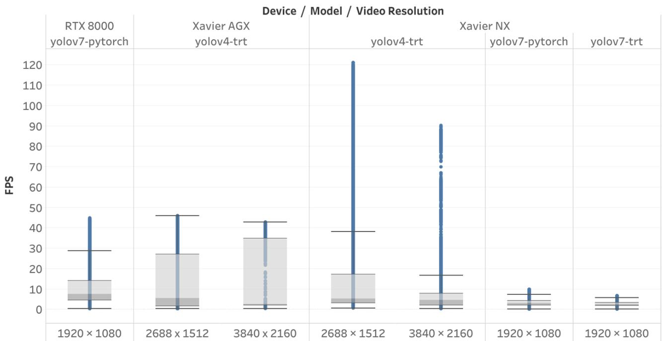
Figure 7. Inference speed per device, detection model, and video resolution.
