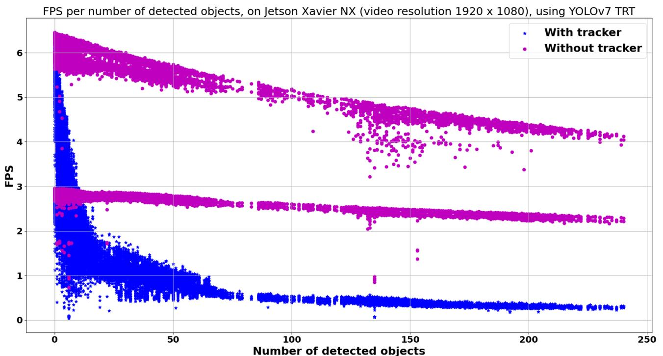
**Figure 11.** Inference speed (in FPS) per number of detected objects, on Jetson Xavier NX, with an input video resolution of  $1920 \times 1080$ , using the TRT version of the YOLOv7 object detection model, when including or excluding the tracker.
