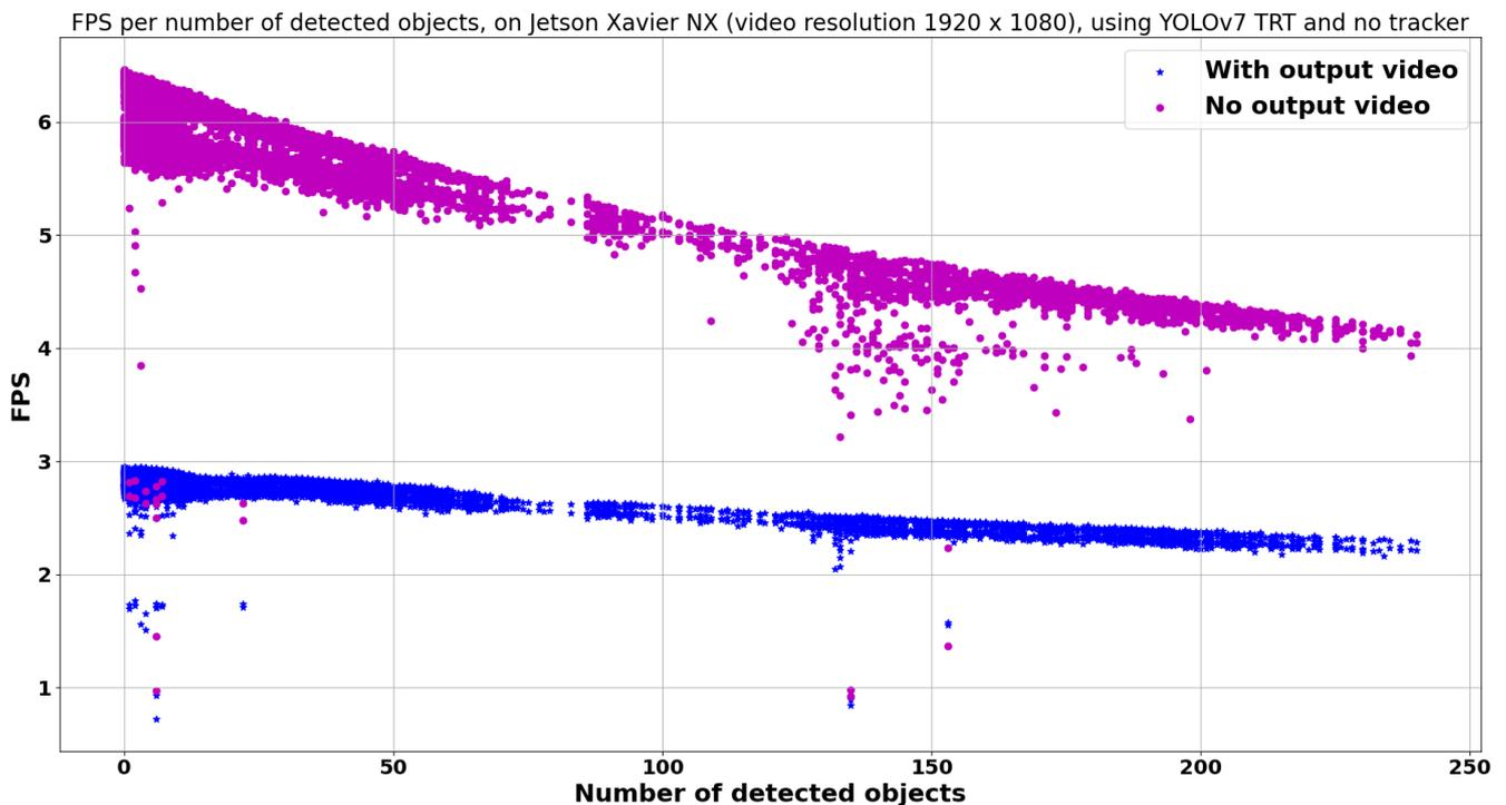
**Figure 12.** Inference speed (in FPS) per number of detected objects, on Jetson Xavier NX, with an input video resolution of  $1920 \times 1080$ , using the TRT version of the YOLOv7 object detection model, with no tracker, when including or excluding the saving of the video output.
