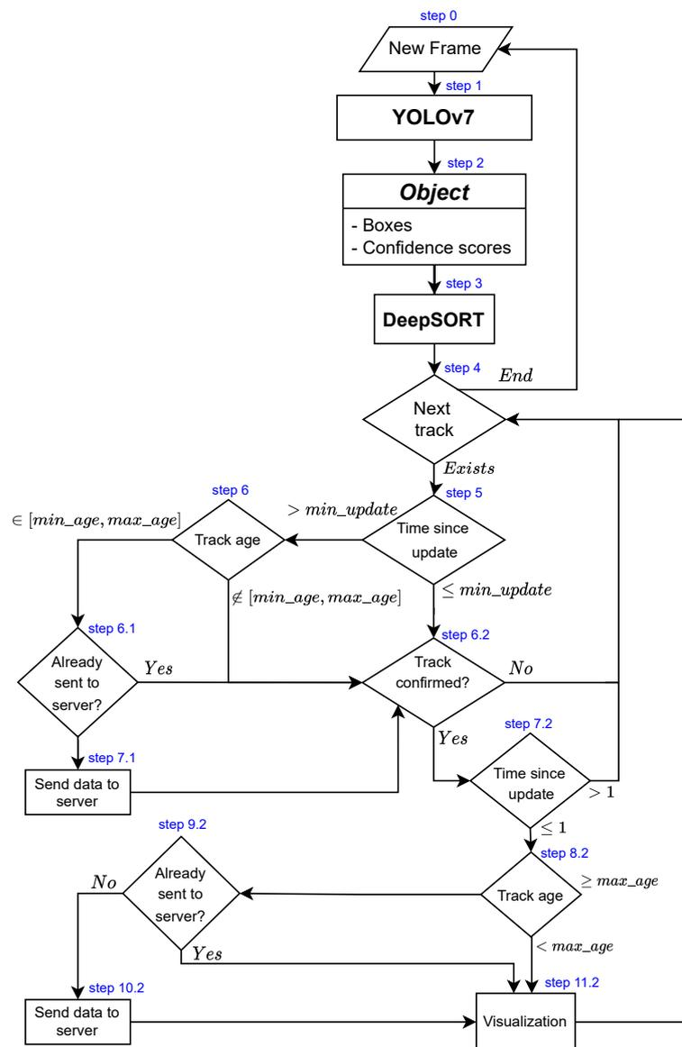
**Figure 4.** The AERO model architecture of the AI module.
