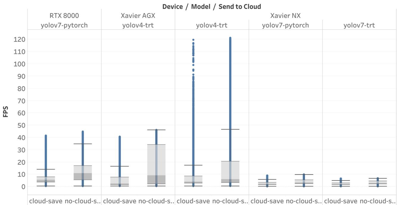
Figure 8. Inference speed per device, detection model, and connection to the cloud.
