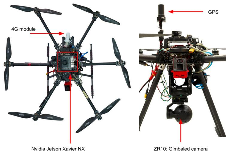
**Figure 2.** Top view of the custom hexacopter.
