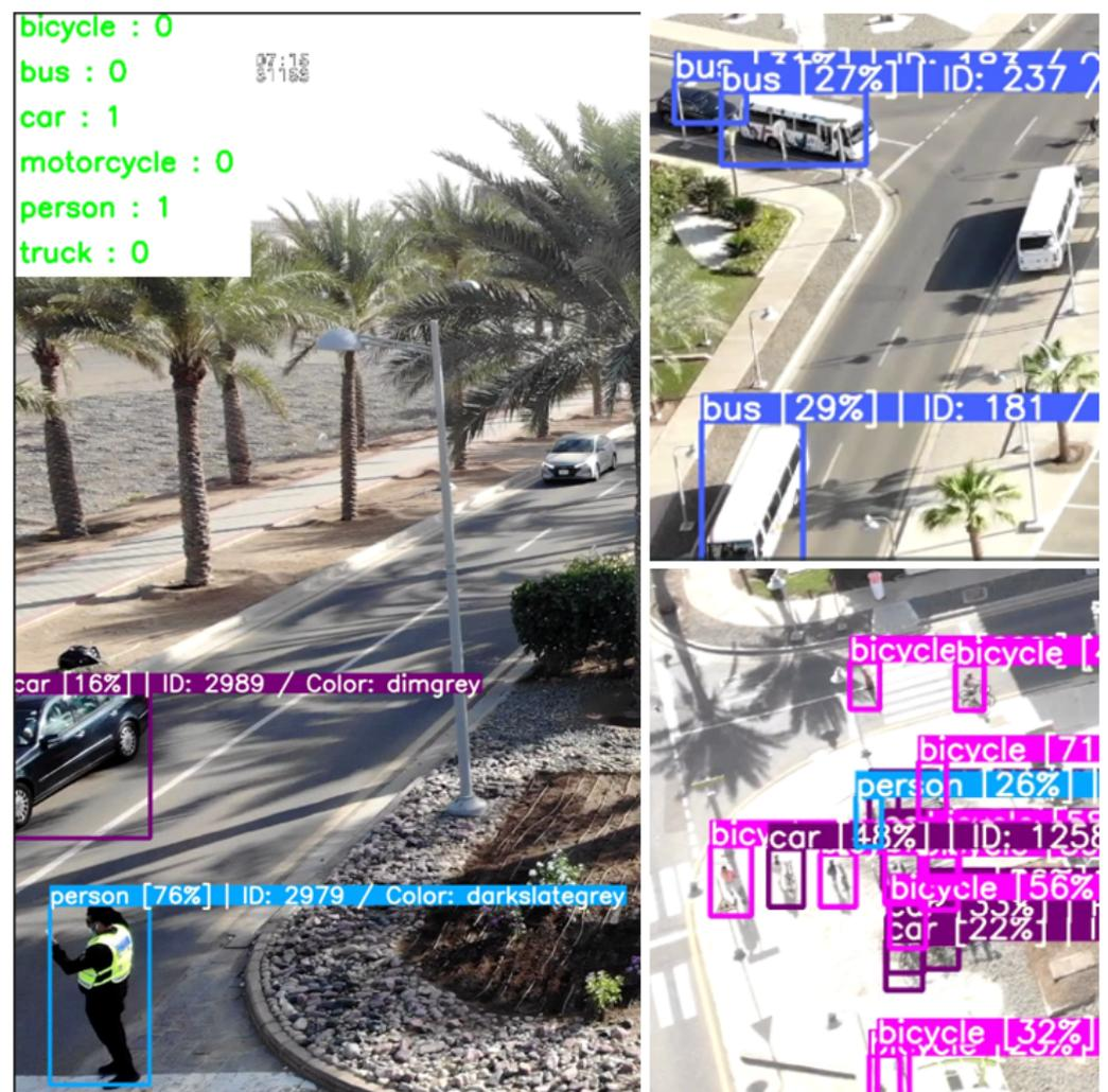
Figure 6. Close view of a sample of the output videos showing various classes, and some false negative and false positive detections.
