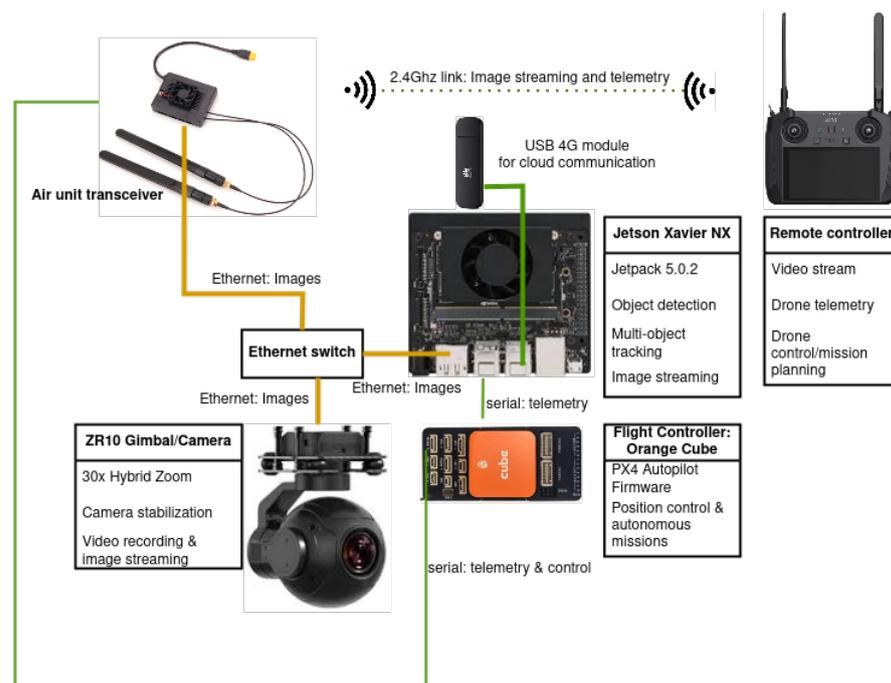
**Figure 3.** UAV onboard electronics.
