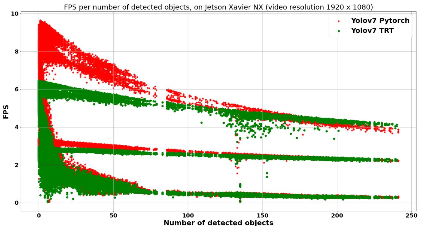
Figure 10. Inference speed (in FPS) per number of detected objects, on Jetson Xavier NX, with an input video resolution of  $1920 \times 1080$ , using the PyTorch and TRT version of the YOLOv7 object detection model.
