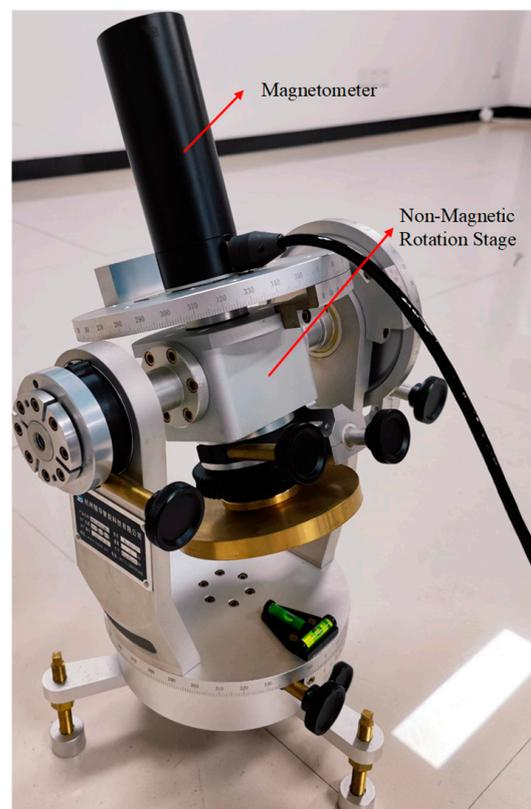
**Figure 5.** Attitude-independent performance verification platform.
