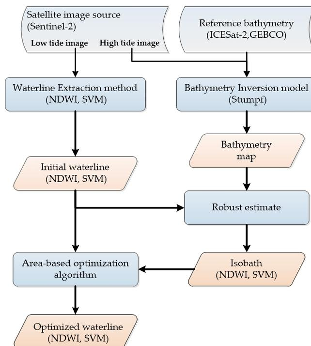
**Figure 2.** Workflow of the proposed waterline extraction approach. The mentioned satellite sensors, waterline extraction methods, and bathymetry inversion models are used in the experiments to demonstrate the proposed approach.
