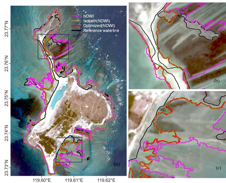
**Figure 6.** JibeI Island's various waterline extraction results based on NDWI method's initial waterline. (a) shows the NDWI initial waterline (purple), its corresponding isobath (green), the final optimized waterline (red), and the reference waterline (black). The background image is Sentinel-2 low-tide image captured on 11 November 2021. (b,c) show two zoom-in regions of (a).
