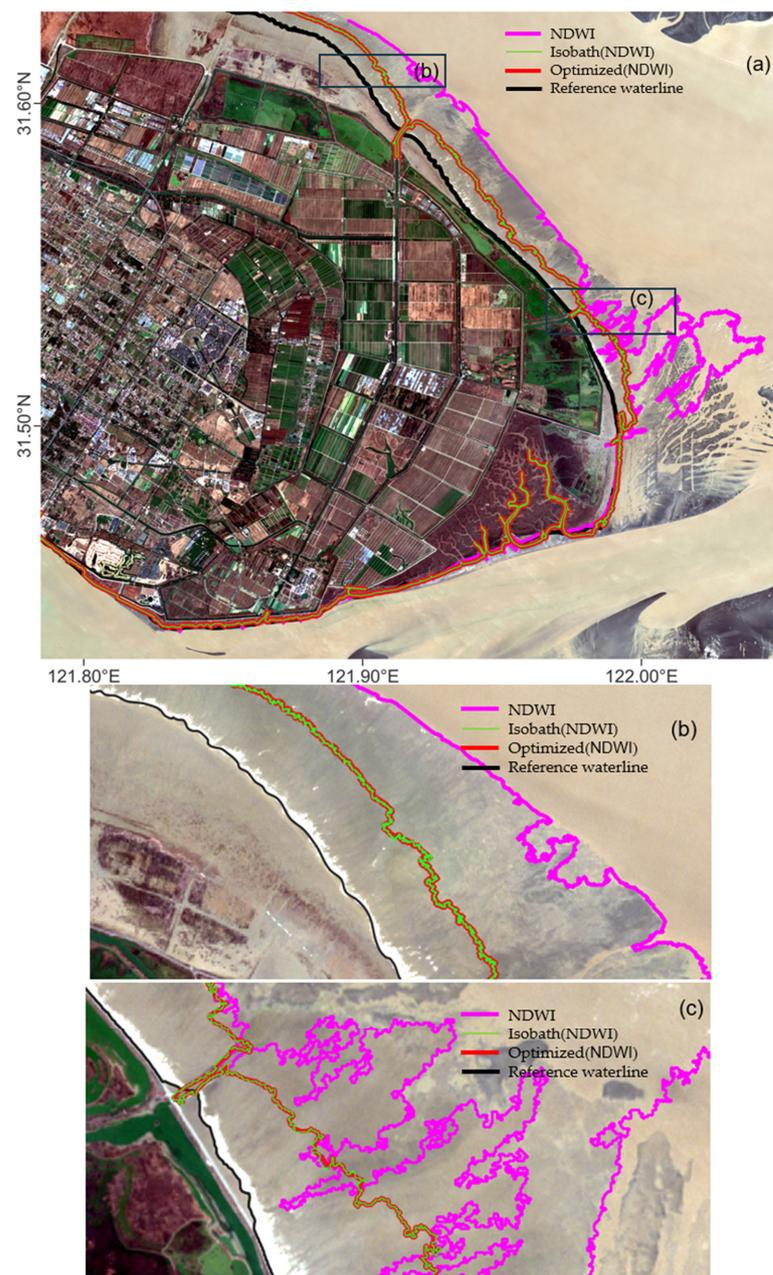
**Figure 8.** Chongming Island's various waterline extraction results based on NDWI method's initial waterline. (a) shows the NDWI initial waterline (purple), its corresponding isobath (green), the final optimized waterline (red), and the reference waterline (black). The background image is Sentinel-2 low-tide image captured on 28 January 2023. (b,c) show two zoom-in regions of (a).
