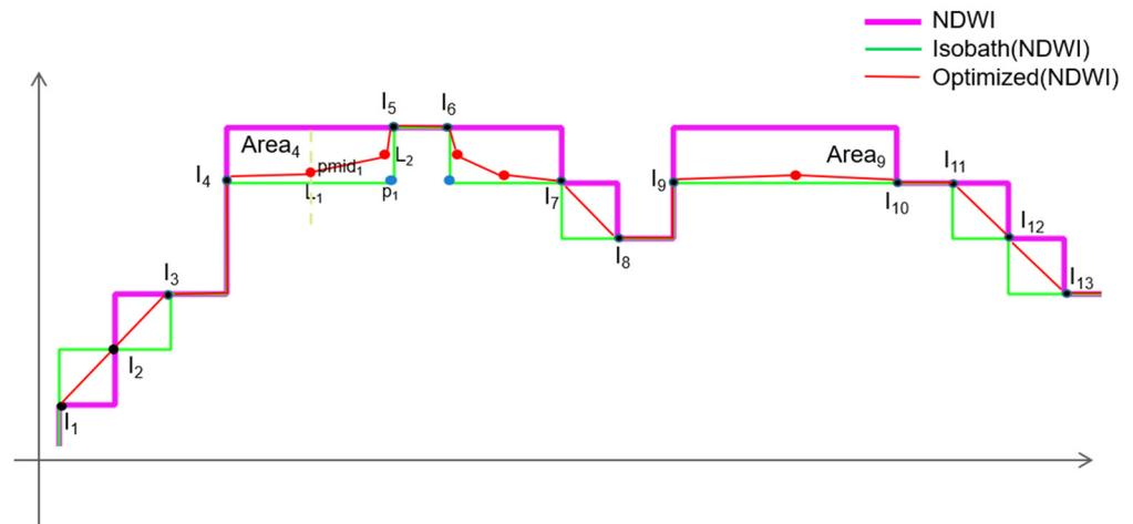
**Figure 5.** The proposed area-based optimization algorithm. The algorithm is to optimize the initial waterline using the estimated isobath and locate a sideline within the two-line siege areas. The green line is the isobath, the purple line is the initial waterline extracted using NDWI method, and the red line is the final optimized waterline.
