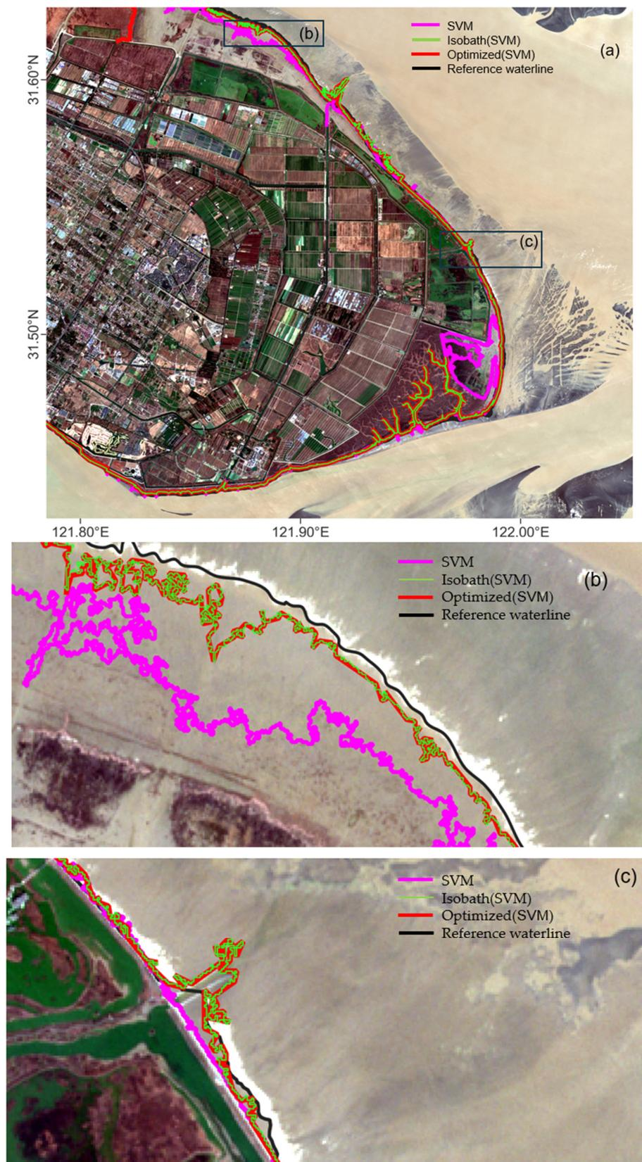
**Figure 9.** Chongming Island's various waterline extraction results based on SVM method's initial waterline. (a) shows the SVM initial waterline (purple), its corresponding isobath (green), the final optimized waterline (red), and the reference waterline (black). The background image is Sentinel-2 low-tide image captured on 28 January 2023. (b,c) show two zoom-in regions of (a).
