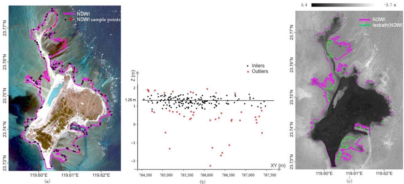
**Figure 4.** Identifying the isobath value of the initial waterline using a robust estimation technique. (a) sample points are extracted along the initial waterline (extracted using NDWI in this case). (b) Finding the robustly estimated isobath value (1.26 m) using samples from the initial waterline (black points are inliers, and red points are outliers). (c) The initial waterline and its corresponding isobath are superimposed on the bathymetry inversion map.
