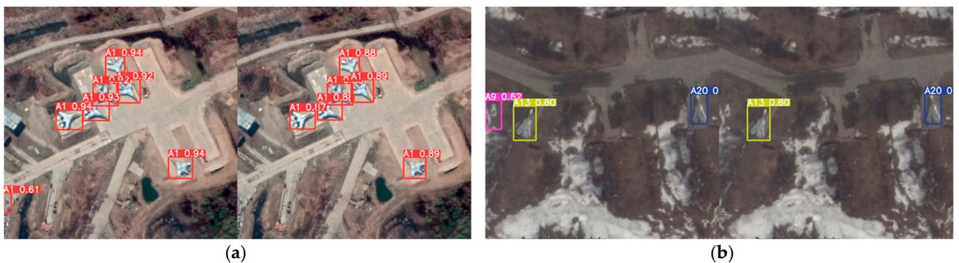
**Figure 7.** Examples of using our network and YOLOv5n to test the same image in MAR20. (a): YOLOv5n, and which has misjudged aircraft targets; (b): our network.
