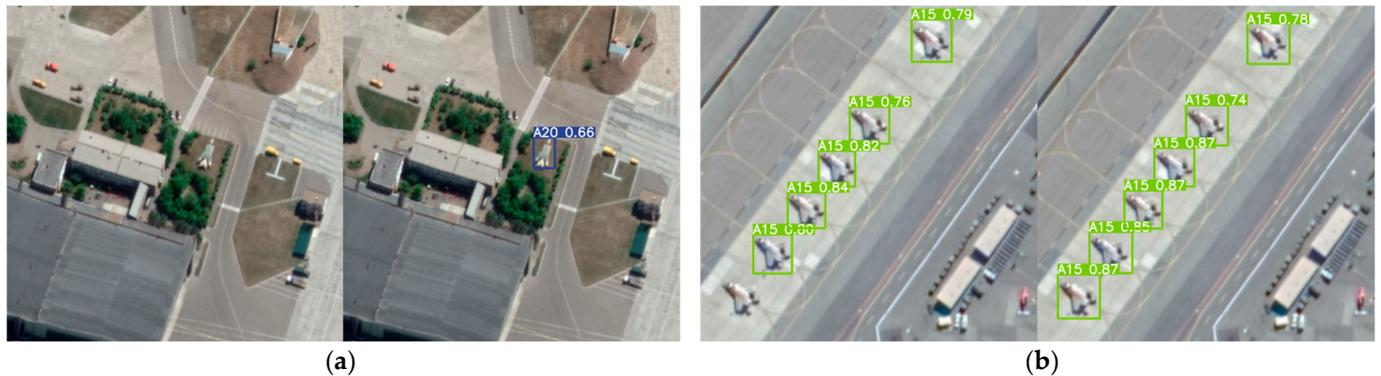
**Figure 8.** Examples of using our network and YOLOv5n to test the same image which have less obvious features in MAR20. (a): YOLOv5n, and which has missed aircraft targets; (b): our network.
