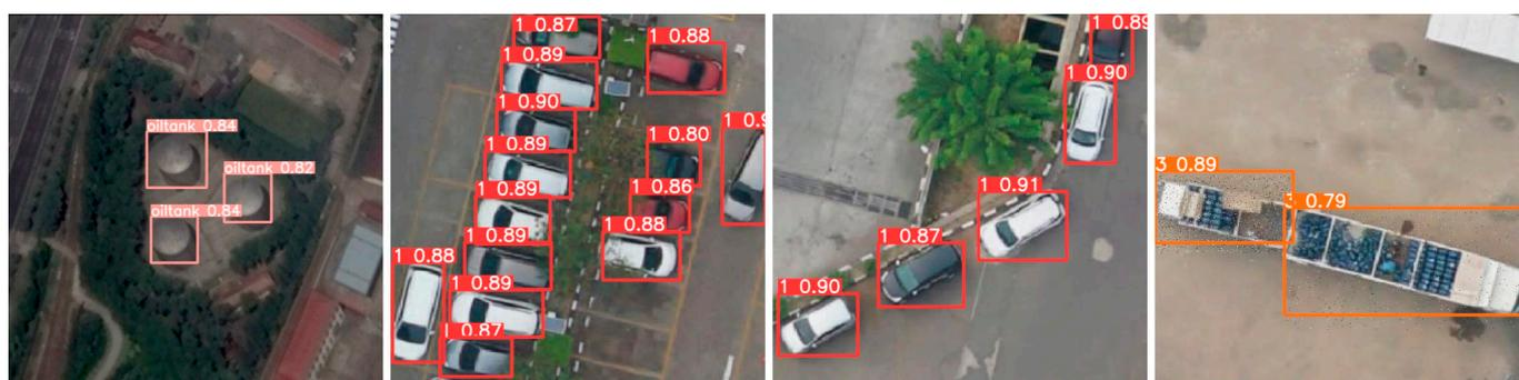
**Figure 9.** Examples of generalization experiments on oil tanks, cars and trucks.
