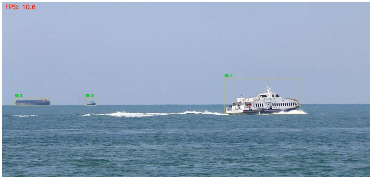
**Figure 19.** Object tracking applied to data from Singapore Maritime dataset [65]. The yellow squares show detected objects that the algorithm is tracking and the green texts show a unique ID given to each object.
