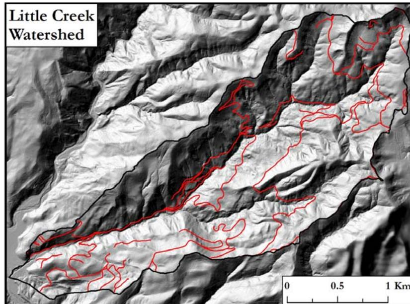
Road edges were well-defined in the LiDAR-derived layers and enabled an accurate digitizing of centerline location. Ninety-five percent of the LiDAR-derived road (3.8 km of 4 km) was digitized within 1.5 m normal to the field-surveyed centerline (Figure 6). The remaining five percent of the road length (0.2 km) was located further than 1.5 m from the surveyed centerline, though the maximum separation between the field-surveyed and digitized centerline did not exceed 2.0 m.
