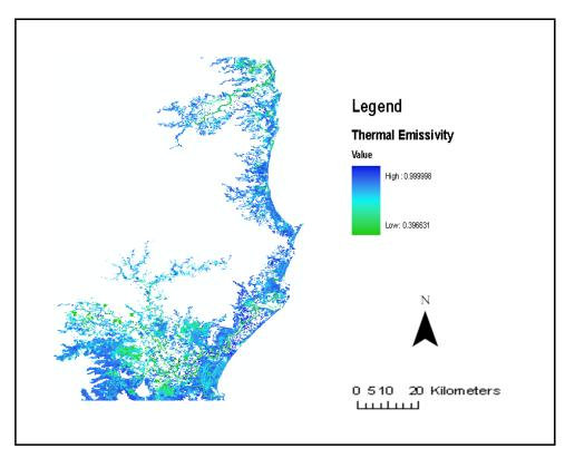
Figure 9. Thermal emissivity values for the wetland classes.
