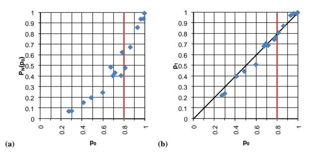
**Figure 6.** Relation between the percolation probability  $P_N(p)$  and the occupation probability p (**a**), and occupation probability values before  $(p_0)$  and after the scaling  $(p_1)$  for the GEOtop data (**b**).
