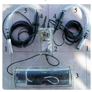
**Figure 2.** Overview image of the radio-transmission underwater video surveillance system for simultaneous recordings of multiple cameras and live viewing on land. It consists of two cameras (1) (board cameras in this figure) connected to two transmitters in a separate housing (2). The back lid of the housing has two cable glands for the antenna cables (3) and one for the power supply cable. The single-battery pack housing is not shown.
