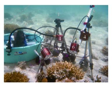
A variety of filters can be used for specific demands. UV- and IR-cut-off filters used during daylight more reliably reproduce color, while an IR-passing filter used during daylight (blocking the visible light), in combination with the IR-light system, provides better insight into the dark regions of highly bright/dark contrasted areas (e.g., interstices of a branching coral).
