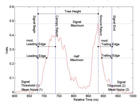
Figure 3. Example of a GLAS waveform and corresponding waveform metrics.
