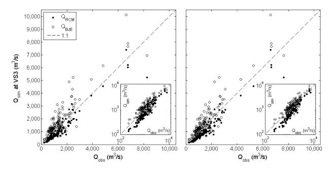
If we compare the observed and simulated discharge considering only ERS-2 altimetry data, RCM works better for VS2 (ERS-2) with RMSE, RRMSE and RE errors lower than the ones computed for VS3 (ERS-2).
