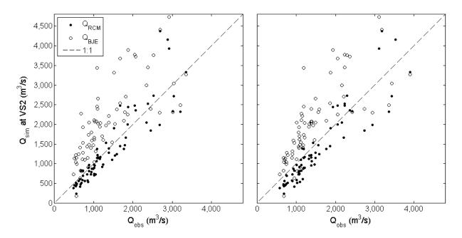
**Table 5.** VS2 and VS3: comparison between the discharge derived from RCM and the empirical equation derived by Bjerklie *et al.* (2003) and the ones observed at Sermide and Pontelagoscuro sections (RMSE = root mean square error; RRMSE = relative root mean square error; NS = Nash Sutcliffe efficiency; RE = relative error)
