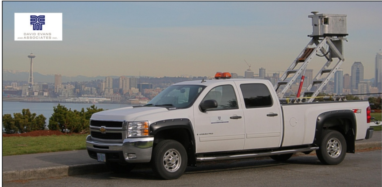
Figure 1. Example of a mobile laser scanning (MLS) system (TITAN, courtesy of DEA).
