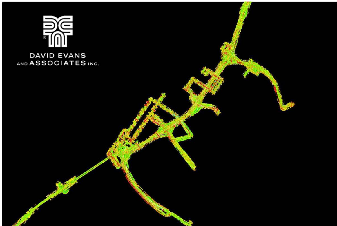
Figure 8. Plan view of a section of MLS data obtained for several arterial roads for the Columbia River Crossing Project, a comprehensive industrial, residential, and infrastructure redesign centered on the I-5 Bridge crossing the river. (Courtesy of DEA).
