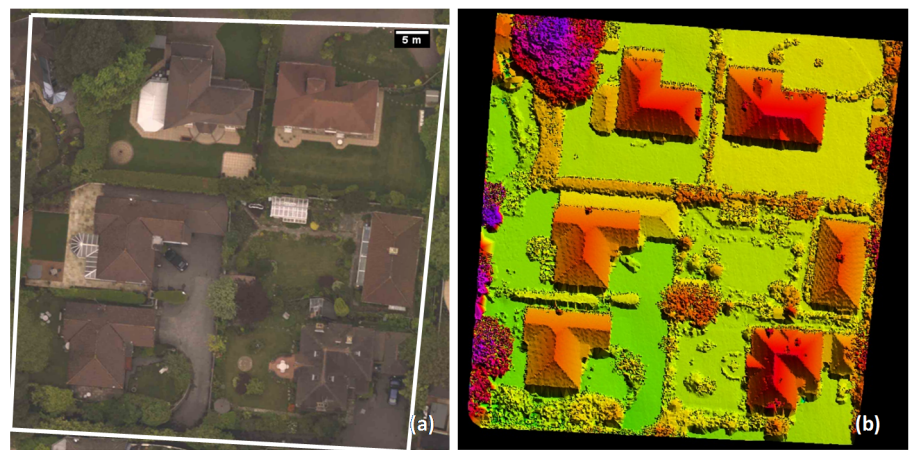
Figure 8. 3D perspective view of segmentation results for the interest area: (a) with FWF physical backscattering information (b) without FWF physical backscattering information.
