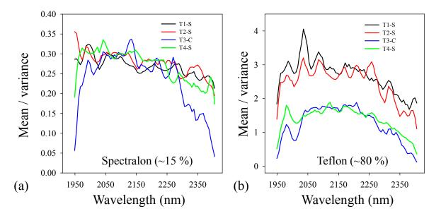
**Table 3.** Average values of mean/variance (1948–2404 nm) from a bright (teflon) and dark (spectralon) target, indicative of the relative amounts of noise in each image. Note smaller values represent greater amounts of noise.
