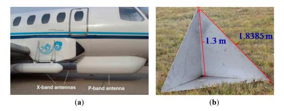
Figure 1. (a) Antennas mounted under the aircraft body; (b) Corner reflector deployed in the calibration site.
