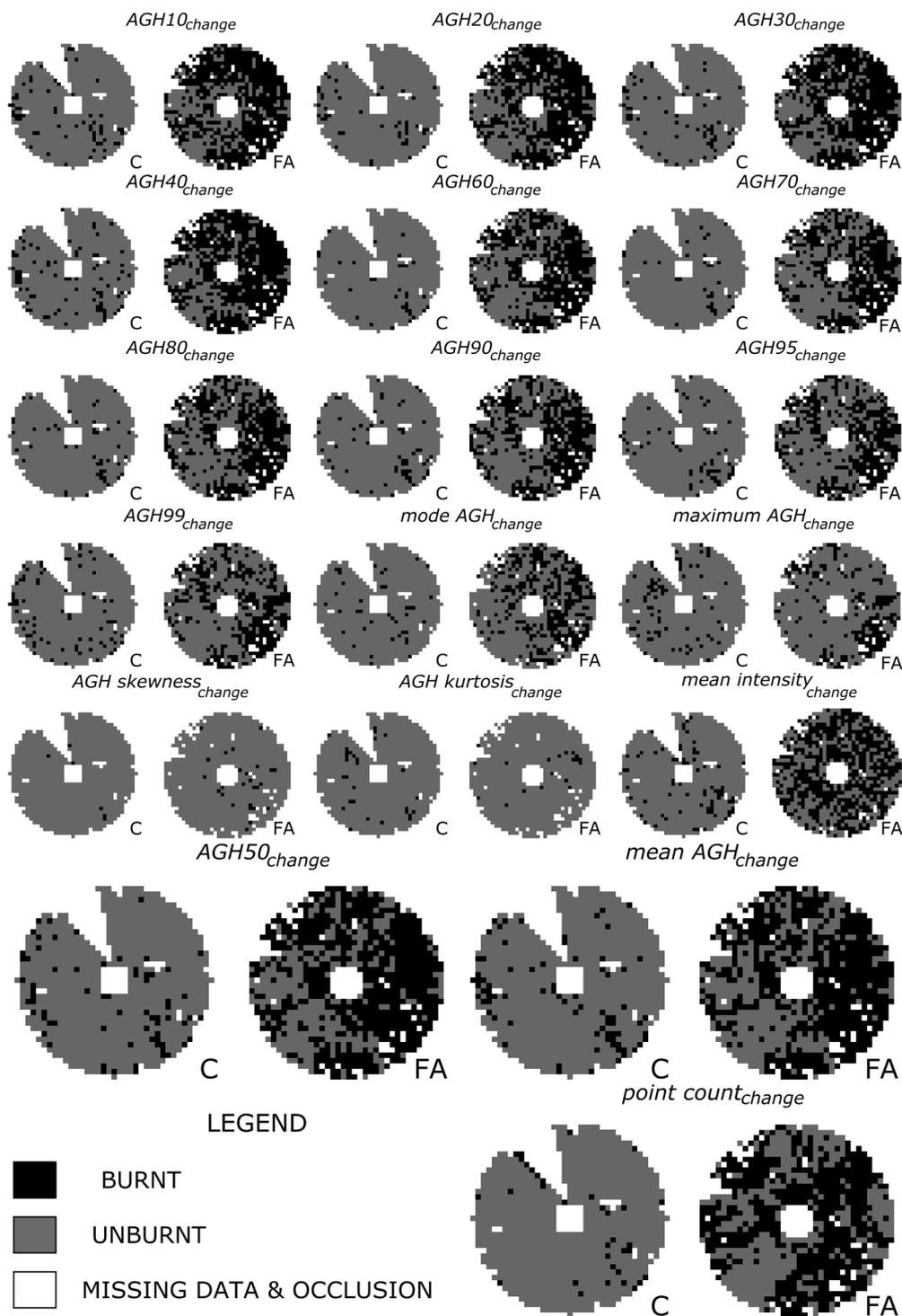
**Figure 6.** Spatial distribution of change detected by the various TLS-derived metrics in the control (C) and fire-altered (FA) plot. Blank areas correspond to occluded voxels or missing data. Areas of no change (grey) were calculated as having values within  $\pm 1.64 \times \sigma$  of the  $\mu$  from the control plot.
