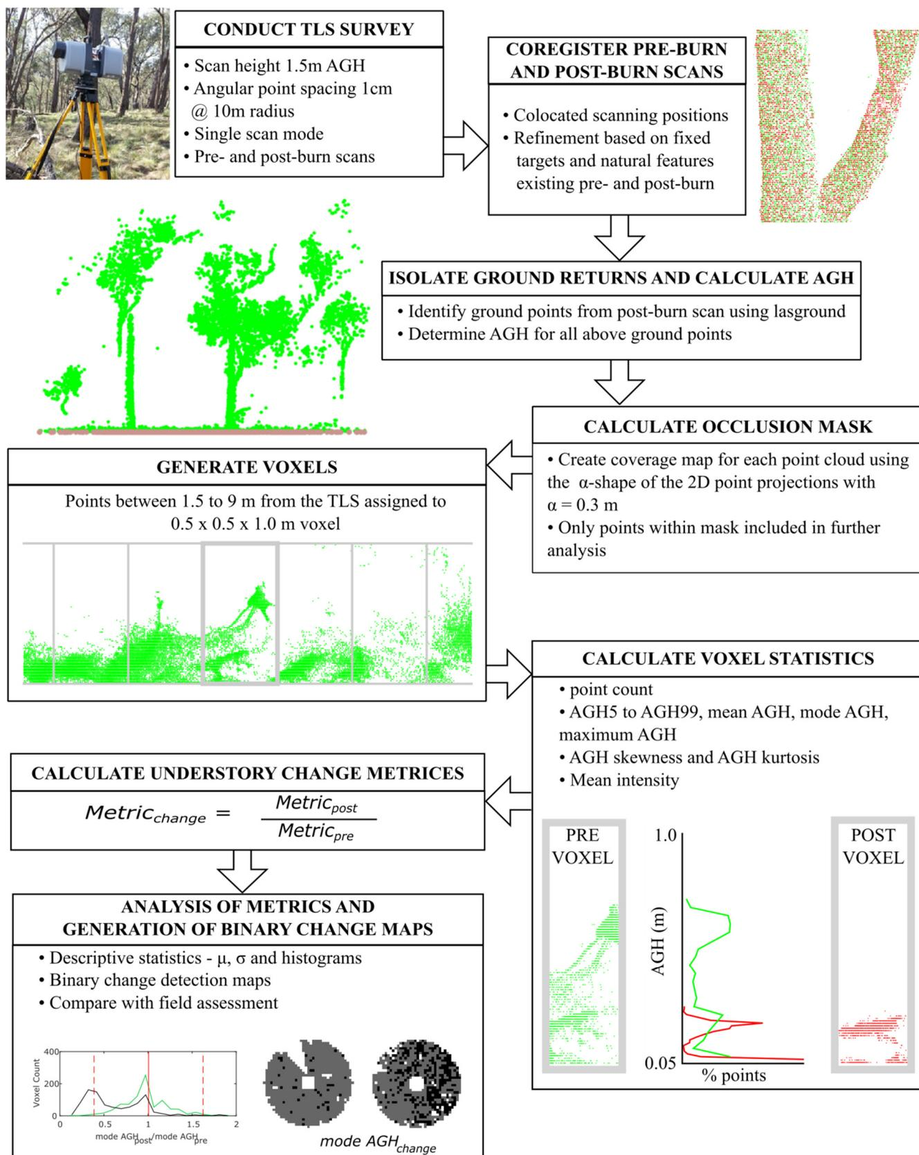
**Figure 2.** The work flow of the TLS data processing for deriving the understory change detection metrics.
