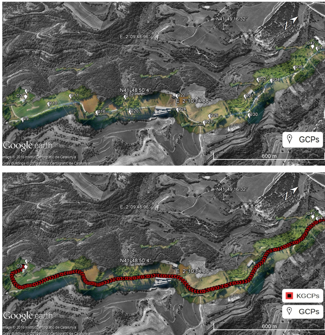
Figure 3. Ground control configuration for the analysed corridors: top , GCP set for conventional corridor; bottom , the mapKITE corridor with two GCPs at the beginning and two more at the end and one KGCP per image.
