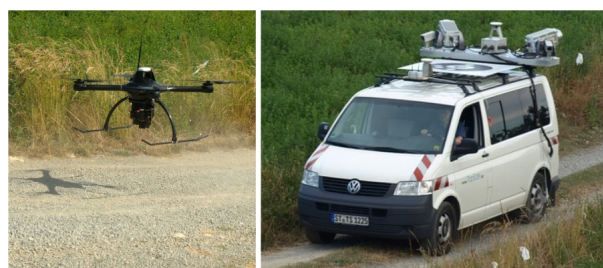
Figure 1. Unmanned aircraft and terrestrial vehicle used in the mapKITE Test Campaign in June 2016. The optical target is seen on the top of the van.
