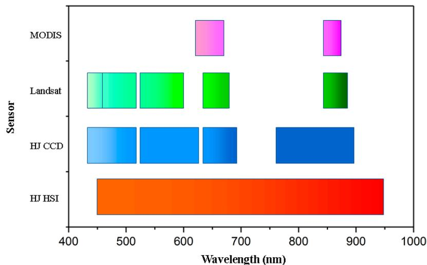
**Figure 3.** The spectral distributions of HSI (115 bands) versus CCD, Landsat 8 and MODIS in the 400–1000-nm range. Each color means one type of sensor, and each block means one band of the corresponding sensor.
