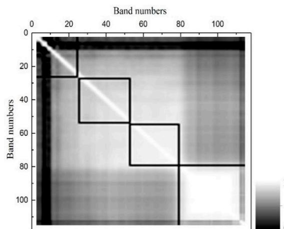
**Figure 4.** The correlation between hyperspectral bands (the darker the tone, the lower is the absolute value of the correlation between bands.) and their separation into 4 groups according to their correlation with 4 multi-spectral bands.
