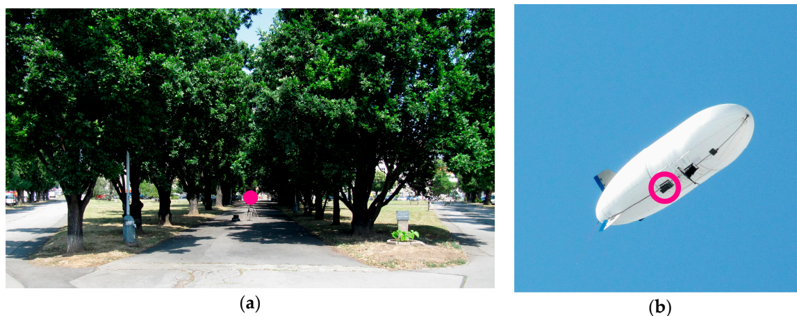
Figure 8. The selected measurement scenario at Fleming Square in Prague, the Czech Republic: (a) location of the receiver marked by the magenta dot; (b) UAV during a flight, the Tx antennas placed on the 3D positioner are marked by the magenta circle.
