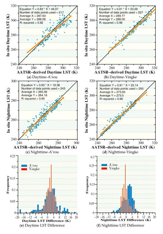
**Figure 2.** Comparisons between AATSR-derived LST and in situ LST at A'rou and Yingke site for 2007–2011: (**a**) daytime comparison at A'rou site; (**b**) daytime comparison at Yingke site; (**c**) nighttime comparison at A'rou site; (**d**) nighttime comparison at Yingke site; (**e**) daytime LST differences for each site; (**f**) nighttime LST differences for each site.
