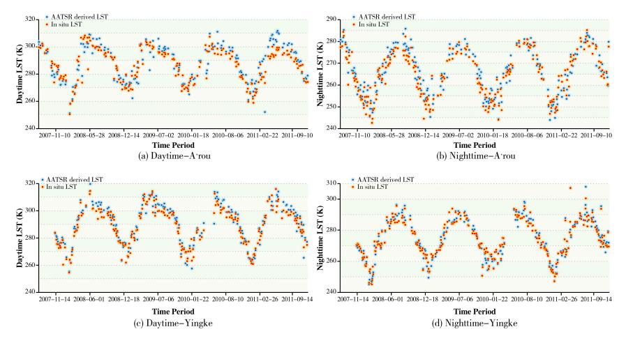
**Figure 3.** Annual phase comparison results between AATSR-derived LST and in situ LST at A'rou and Yingke site for 2007–2011: (**a**) daytime comparison at A'rou site; (**b**) nighttime comparison at A'rou site; (**c**) daytime comparison at Yingke site; (**d**) nighttime comparison at Yingke site.
