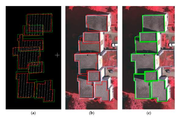
**Figure 7.** Compensation of occlusion effects: (**a**) lack of ALS points due to height differences and occlusions (marked in yellow); (**b**) roof outlines extracted from ALS; (**c**) edges refined by the information extracted from the aerial image.
