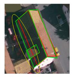
**Figure 4.** Matching line pair (marked in yellow) detected with increasing matching threshold; ALS-based lines (red), image-based lines (green).
