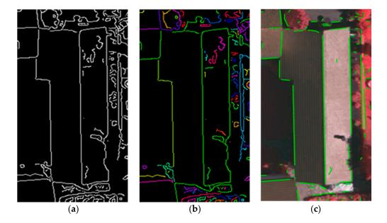
**Figure 3.** Straight line extraction: (**a**) boundary image derived by Canny edge detector; (**b**) connected component labelling; (**c**) pixels connected into straight line segments.
