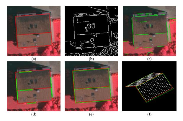
**Figure 2.** Refinement process: (**a**) input wireframe model projected into image space; (**b**) initial result of edge detection; (**c**) detected straight lines; (**d**) correspondence matching; (**e**) refined wireframe model (green) compared to input model (red); and (**f**) comparison of building models in 3D space before and after refinement.
