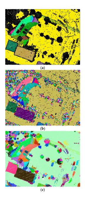
**Figure 3.** Results of internal steps in the step-wise point cloud segmentation: (**a**) Intermediate result after the process of the region growing (RG) with RANdom SAmple Consensus (RANSAC) step. The scattered points are rendered in black; (**b**) Intermediate result after the process of the initial patch construction; (**c**) The result of the step-wise point cloud segmentation.
