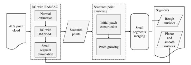
Figure 2. The flowchart of the step-wise point cloud segmentation.
