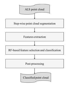
Figure 1. The proposed framework for airborne laser scanning (ALS) point cloud classification.
