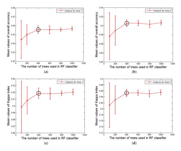
**Figure 10.** The variation tendencies of mean overall accuracy values and standard deviation values of overall accuracy and Kappa coefficient under different settings of  $N_{tree}$ ; (**a**,**b**) are for Area 1 and Area 2 respectively; (**c**,**d**) are for Area 1 and Area 2 respectively.
