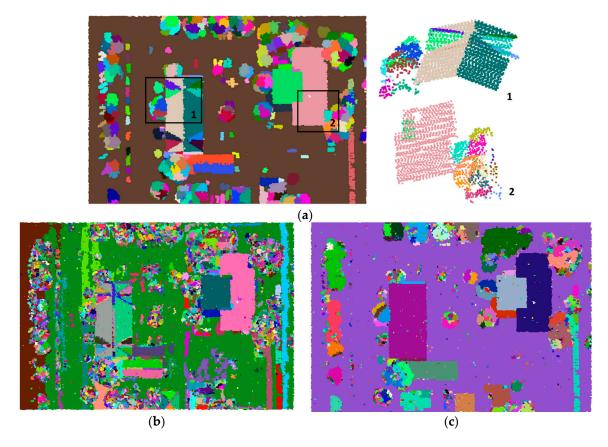
**Figure 7.** Comparison of our segmentation method with the RG methods presented in Point Cloud Library (PCL): (a) The result of our method; (b) The result of the RG-based plane segmentation; (c) The result of the RG-based smoothness segmentation.
