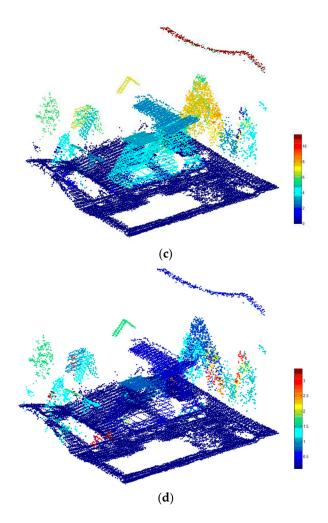
**Figure 5.** Segment-based features for 3D-point clouds classification, (**a**) horizontal projection area ratio  $PR_h$ ; (**b**) eigenentropy  $\lambda_e$ ; (**c**) relative elevation  $H_r$ ; (**d**) slope  $O_{sl}$ .
