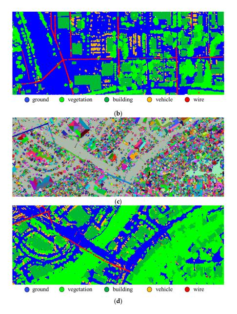
**Figure 16.** The results of the proposed classification framework for areas Area 1 and 2, (**a**) is the segmentation result of Area 1; (**b**) is the classification result of Area 1; (**c**) is the segmentation result of Area 2; (**d**) is the classification result of Area 2.
