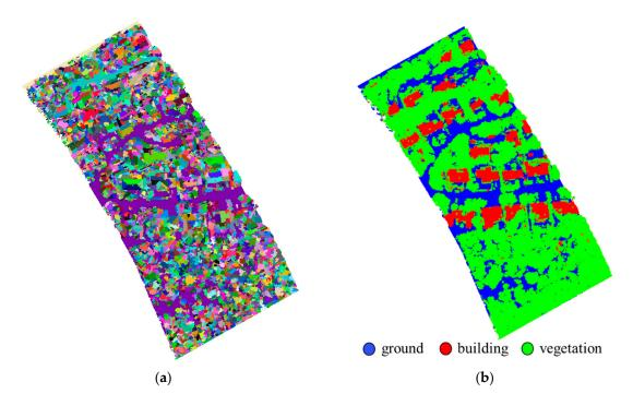
**Figure 17.** The results of the proposed classification framework for Area 3, (**a**) is the segmentation result of Area 3; (**b**) is the classification result of Area 3.
