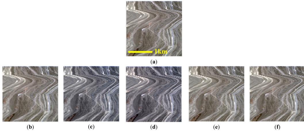
**Figure S3.** Reconstructed HSI of different super-resolution methods, the images are shown in RGB (band 35, 25, 15). The sub-image with size  $128 \times 128 \times 162$  is cropped from *Cuprite-1* of AVIRIS data. (a) Original sub-image, (b) result of sparseFU, (c) result of SUN, (d) result of BayesSR, (e) result of SSR, (f) result of CNMF.
