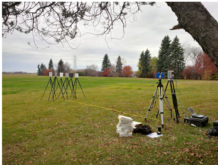
Figure 2. A photograph showing the setup of the experiment for one of the field tests. The two scanners are on the right side of the photograph and the six diffuse reflectance targets are in the upper left portion.
