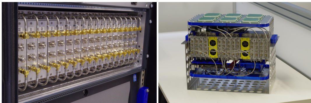
Figure 9. Left: RF front-end of the SPIR Instrument. The control and recording system is implemented in a standard industrial PC. Right: SPIR-UAV instrument to be flown on-board a UAV for the remote sensing of the sea-surface ice of the arctic.
