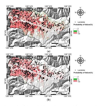
**Figure 10.** Maps showing slope failure probability predicted using **(a)** fuzzy PEM with reduced COV and **(b)** Monte Carlo simulation with reduced COV.
