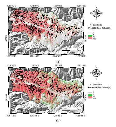
**Figure 11.** Maps showing slope failure probability predicted using fuzzy PEM with (a) fuzzy numbers of mean  $\pm 1~\sigma$  and (b) fuzzy numbers of mean  $\pm 3~\sigma$ .
