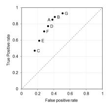
**Figure 7.** ROC graph comparing the analysis results. A: fuzzy PEM, B: probabilistic analysis (Monte Carlo simulation), C: deterministic analysis, D: fuzzy PEM with reduced COV, E: probabilistic analysis with reduced COV, F: fuzzy PEM with  $\pm 1$   $\sigma$ , G: fuzzy PEM with  $\pm 3$   $\sigma$ .
