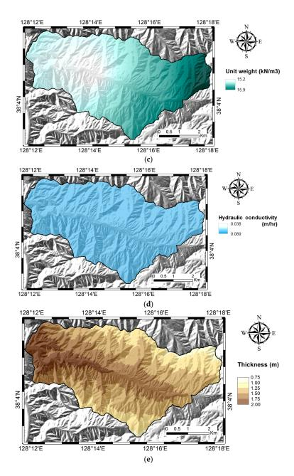
**Figure 4.** The distributions of (a) friction angle, (b) cohesion, (c) unit weight, (d) hydraulic conductivity, and (e) soil thickness.
