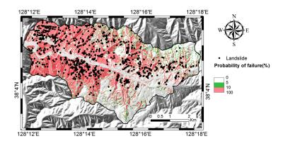
Figure 8. Map showing slope failure probability predicted using Monte Carlo simulation.
