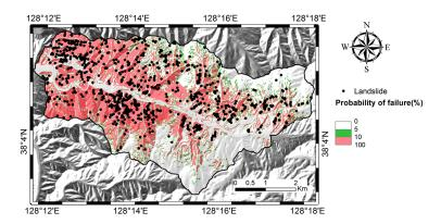
Figure 6. Map showing slope failure probability predicted using fuzzy PEM.
