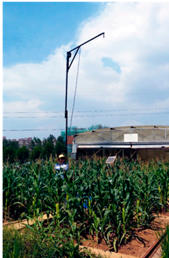
Figure A3. A hand-held mobile system for measuring canopy spectral reflectance. A 2 m horizontal boom is mounted on a 4 m vertical pole to support an Analytical Spectral Devices (ASD) FieldSpec 3 spectrometer to measure the canopy optical spectra in the nadir direction.
