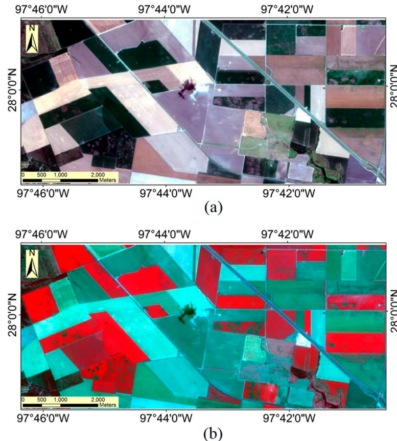
Figure 3. Sentinel-2A multispectral instrument (MSI) image for the study area. (a) True color image; (b) color infrared (CIR) composite image.
