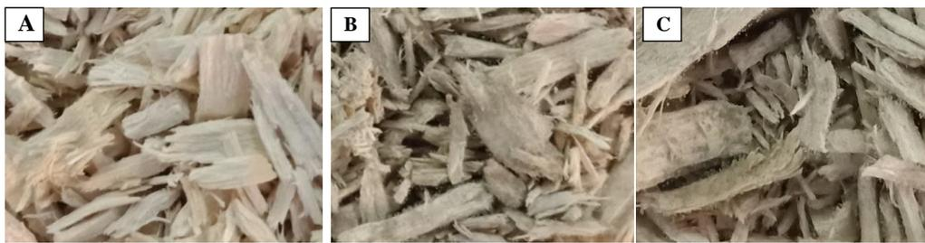
**Figure 1.** Typical samples observed under the sunlight. (A) negative control; (B) inoculated sample after incubation for seven days at 23 °C and 82% humidity; (C) inoculated sample after incubation for seven days at 30 °C and 88% humidity.
